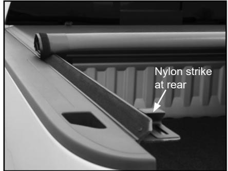
B. Close tailgate slowly, top of tailgate should fit snug under rear bar. If cover impedes normal tailgate operation, raise side rails by: loosening rear clamps, adjusting side rail up and then tightening clamps. If there is a gap between tailgate and cover, adjust side rails lower.
