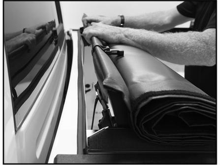
C. Slide left tension adjuster until it engages under side rail (see Step 5F). Push bar back and forth to line up holes. Do not turn adjustment wheel. Insert bolt from top then secure with washer and nut from bottom.
