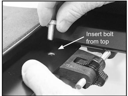
D. Hold bolt at top and tighten nut under side rail. Repeat Step 5C and 5D for right tension adjuster.
