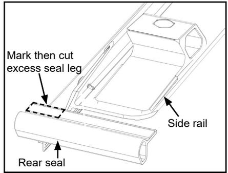
C. Peel paper back, align and adhere seal to end of side rail.
