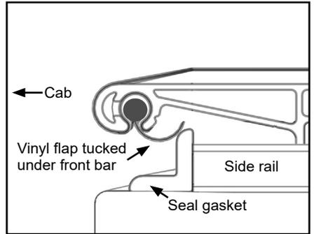
F. With the tension adjuster's support tab under the side rail, tighten bolt (left loose earlier) under front bar on each tension adjuster.
