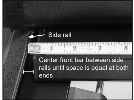
**NOTE:** Before tightening, ensure the vinyl flap is tucked under front bar.
