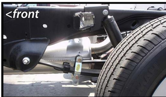
Front shackle install in top hole
