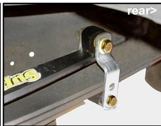
SSA12 square shackle to rear SSA8 has beveled shackle to rear
