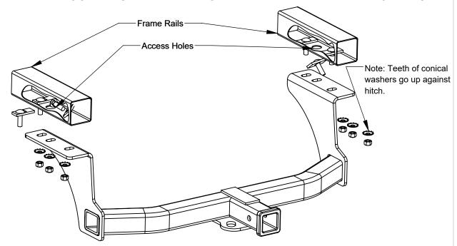
Note: To ease hardware installation enlarge access holes with die grinder
