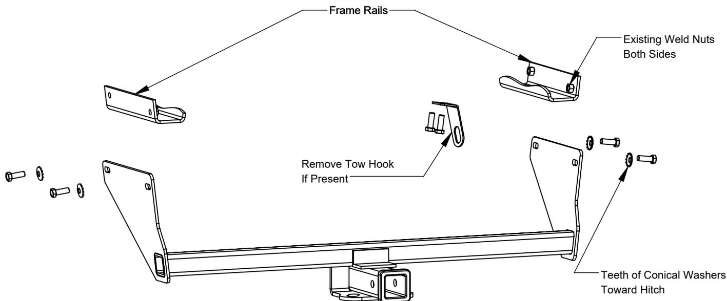
1. Remove the stickers covering the mounting holes on the outside of frame rails.
