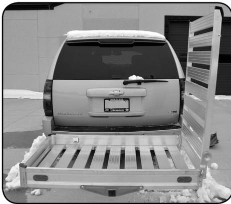
Ramp Folds down and into carrier
