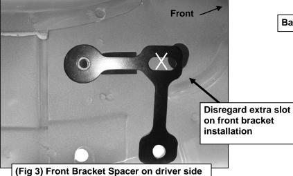
Spacer installs between the body panel and front Bracket only
