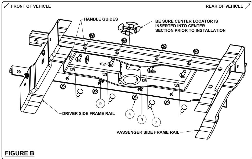
Slide this cross arm as far rearward as possible. Insert the second cross arm in the same manner as the first only positioned so the holes now face the rear of the truck. Do not slide this cross arm rearward yet.
