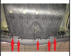
Fishwire (2) 7/16" carriage bolts and (2) CM-SP2 spacers through the vehicle access holes to the attachment holes on each side. See FISHWIRE DIAGRAM below.
