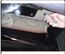
5. Torque all 12mm hardware to 86 ft-lbs. Torque all 7/16" hardware to 70 ft-lbs.
