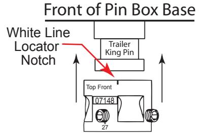
Slide the locking collar over the trailer king pin. Before tightening allen-head screws, rotate the collar so that the white line of the locator notch on the front of the collar is in the exact center of the front of the king pinbox. Tighten each of the allen-head screws evenly, **making sure the allen head screws rest on the bottom lip of the trailer king pin.** Firmly seat the allen-head screws flush with the surface of the collar. If screws are not flush, loosen and re-tightened evenly.
