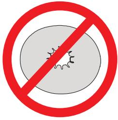
Remove the **Fifth Wheel Lube Plate** or **Lubrication Disk** from around your King Pin, (if your trailer is equipped with one.)
