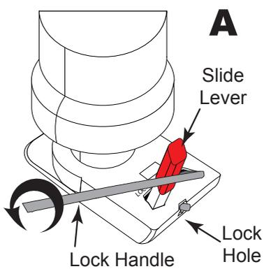
With the lock handle in front of the slide lever, twist curved end through lock hole in the base.
