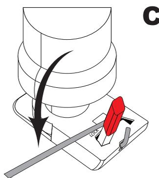
Lower the handle to the bed of the truck. This will prevent the sliding lever from moving from the locked position
