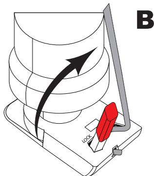
To achieve positive lock, lift the lock handle up and move behind the slide lever.
