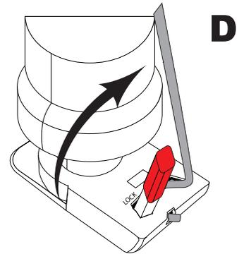
To Remove, lift the handle back up and over the slide handle.
