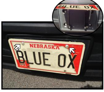
2. Install the license plate onto the license plate bracket, using two (2) #10-24 screws, in the upper two (2) plastic inserts.
