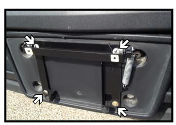
Remove the existing license plate. Install the license plate bracket into the factory holes with four (4) 1/4"-20 screws.
