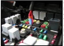
under hood fuse box. Remove the large plastic fuse box cover and remove the high amperage (e.g. 50 amp) fuse. Confirm that the colored connectors on the Fuse ByPass
