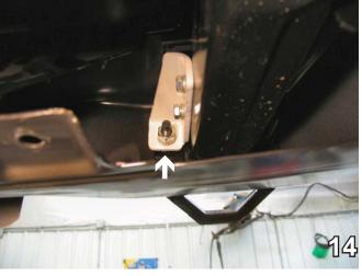
14. Remove the existing bolt, 12MM hex nuts (reference #9 on page 5 of this document) and replace fascias according to the directions on the previous pages. This procedure is done on both sides of the vehicle, the passenger's side is shown.
