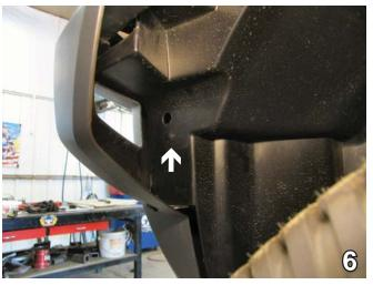
6. On the backside of the lower fascia, remove one push pin from the lower front fascia. Set the push pins aside as they will need to be re-installed. This procedure is done on both sides of the vehicle, the driver's side is shown.
