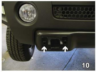
10. Remove the metric bolts from the tow hook bracket, using a 18MM Socket. Set aside as they will be used for the baseplate installation. Pull the lower front bumper fascia forward and set carefully aside as it will need to be re-installed.
