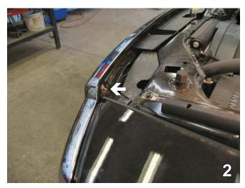
The upper and lower front fascias will need to be removed for this baseplate installation. Using a 10MM Socket, remove one metric bolt from behind the upper front fascia. This procedure is done on both sides of the vehicle, the driver's side is shown.
