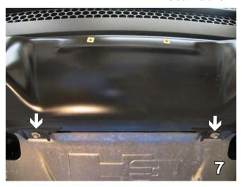
On the bottom side of the lower front fascia, where the belly pan meets the lower front fascia, remove two metric bolts using a 13MM Socket. When the bolts have been removed, set them aside as they will need to be reinstalled.
