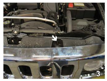
On the front side of the upper front fascia, using a 10MM Socket, remove one metric bolt. Set aside as these bolts will need to be re-installed. This procedure is done on both sides of the vehicle, the driver's side is shown.
