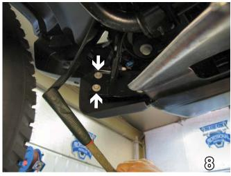
Next you will need to pull back, but DO NOT 8. **REMOVE**, the webbing from the underneath side of the lower front fascia and remove 2 metric bolts using a 13MM Socket. Set these bolts aside as they will need to be re-installed. This procedure needs to be done on both sides of the vehicle, the driver's side is shown.
