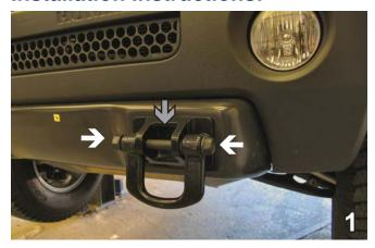
Using a 24MM Socket, remove the tow hooks from the front fascia. Set aside and return to customer as these will NOT be reinstalled on the vehicle. Some models will have bolts to remove with a T-30 Torx socket. This procedure will need to be done on both sides of the vehicle, the driver's side is shown.
