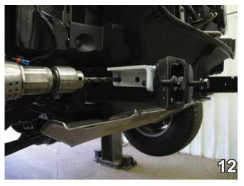
12. Using the baseplate as a template, drill the holes with the 13/32" drill bit, for the baseplate to mount to the frame rail.
