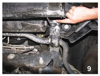
2009 Models: Using a 10MM socket, remove the metric bolt from the impact bar support. Do this on both sides. Set the bolts aside to be reinstalled after the bracket is attached in step 11.
