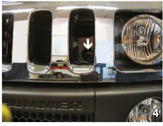
Inside the grill, near the headlight assembly remove one metric bolt using a 10MM Socket. This procedure is done on both sides of the vehicle, the driver's side is shown.
