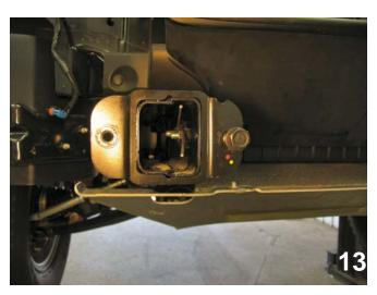
13. Insert the nut plates into the frame rail to align with drilled holes and tighten the 3/8"-16 hex bolts and 3/8" lock washers according to the torque chart on page one of this document. (BE SURE TO USE LOCTITE RED.) This is done on both sides of the vehicle, the passenger's side is shown.
