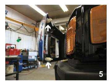
5. Release the clips on the grill and pull forward to remove, set carefully aside as it will be re-installed. There are two clips on each side, this procedure will need to be done on both sides of the vehicle, the driver's side is shown.
