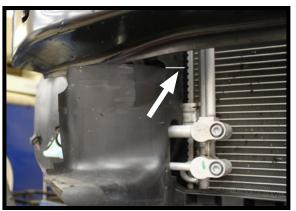
8. Cut straight across on the top of the plastic tab. After the cut has been made, lift up and remove the tab. Do this on **BOTH** sides.
