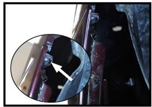
3. Pull the wheel well liner back. Using a Torx 25 remove the screw that is located underneath. Do this on **BOTH** sides of the vehicle.
