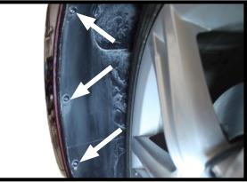
Remove the three (3) screws in the front wheel well area using a Torx 25. Do this on **BOTH** sides of the vehicle.
