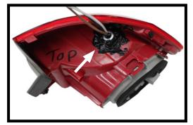
Drill a hole according to the tail light wiring kit instructions.
