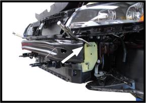
9. Place the baseplate under the bumper centering the slot on the bottom of the baseplate with the existing hole in the bumper. Securely clamp the baseplate into postion. Take extra care on the passenger side not to hit the lines. NOTE: If the horn is in the way, gently bend it outward.
