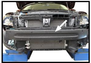
6. Pull the styrofoam bumper padding off and place to the side for reinstallation after the baseplate is installed.
