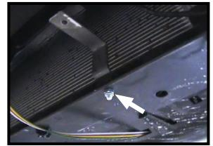
You may place the breakaway bracket anywhere on the vehicle frame. Using a 9/32" drill bit, drill a hole into the frame.
