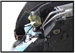
Verify the baseplate is level and install the 3/8"-16 x 1-1/4" hex head bolts, 3/8" lock washers and 3/8" flats washers on the bottom slot. Do this on **BOTH** sides of the vehicle.
