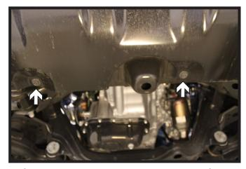
2. Using a 12MM socket, remove the four (4) screws from the belly pan on the underside of the vehicle.
