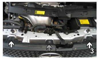
Above the grill, remove the cover. Using a 10MM socket, remove two metric bolts. Using a flat screwdriver, remove push pin from the center (grey arrow). Set cover, bolts and pin aside to be reinstalled later.
