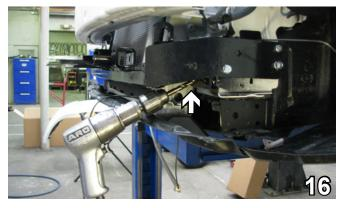
16. Using the 13/32" drill bit, drill at an angle one hole using the baseplate as a template into the front of lower frame support. Do this on both sides.
