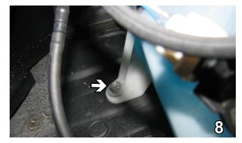
Using a 10MM socket, remove the bolt from between wheel well cover and left side of washer reservoir on the passenger side only. Disconnect all electrical and fluid lines, then remove reservoir and bolt. Set aside for later reinstallation.
