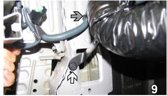
On the driver's side, using a flat screwdriver remove the push pin holding the vent tube. Also pull out the clip (grey arrow) from wire loom. Move the vent tube out of the way. Save the pin to reinstall later.
