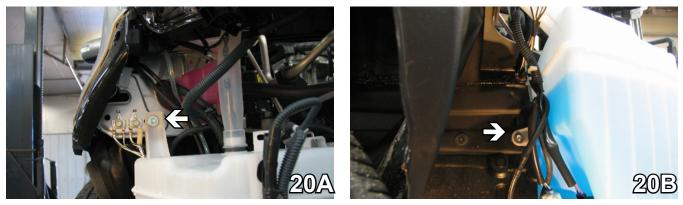
20. Attach top and left washer reservoir with #10-16 x 1" self drilling screws with 1/4" flat washers into frame. Reattach all wires and hoses.
