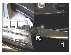
1. Remove the three push pins from the top edge of front grill.
