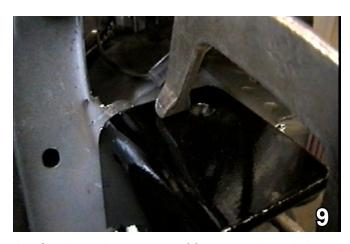
Set baseplate on top of frame ends and clamp in place. Baseplate should be firm against the front of radiator support. Using the baseplate as a template drill three holes with the 13/32" drill bit, both sides.
