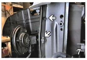
7. Pinch clips together on the back of radiator support and pull air dam forward, both sides and set aside.
