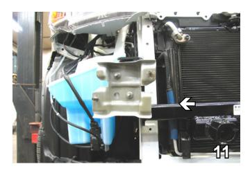
**11.** Wrap the coolant line behind the baseplate with the tubing and two cable ties provided.
