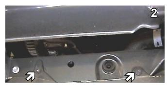
Remove two metric bolts from top edge of fascia's tabs with the 10MM socket. Remove one push pin.
