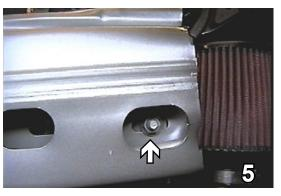
**5.** Using the 12MM socket, remove four metric bolts from metal bumper, pull metal bumper forward and set aside.
