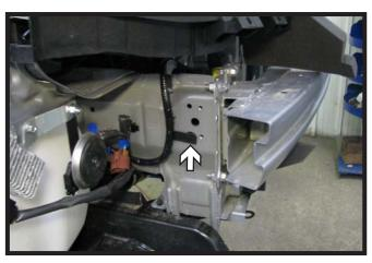
5. On the passenger side, remove the wiring clip and move the wires out of the way.
