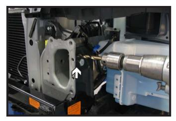
11. Tip the baseplate into position. Install a 1/2"-13 x 1-1/4" bolt with 1/2" flat and lock washers into the existing hole and secure with a 1/2"-13 lock nut on the inside of the frame. Do this on both sides of the vehicle. Level the baseplate and fully tighten both bolts.
