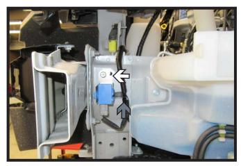
4. On the driver side, using a 10MM socket, remove the bolt from the sensor bracket. Remove the wiring clip and move the sensor and wiring out of the way (gray).
