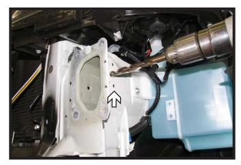
10. If needed, using a 17/32" drill bit, ream the existing hole in the frame as shown. Some models may come with a larger hole and do not need to be reamed. Do this on both sides of the vehicle.
