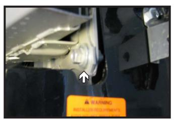
17. Reinstall the metal bumper with the existing bolts. Use two (2) 5/16" washers on bottom as spacers.
