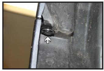
2. In the wheel well where the fascia meets the fender, remove the push pin. Do this on both sides of the vehicle.
