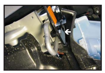
15. On the bottom baseplate hole, insert the spacer tube between the frame and the baseplate. Insert a 3/8"-16 x 2" bolt, 3/8" flat & lock washer and 3/8" lock nut. Do this on both sides of the vehicle.
