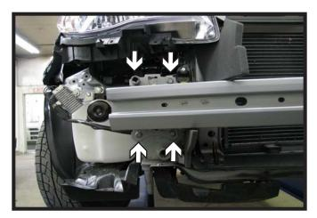
7. Using a 12MM socket, remove the four (4) bolts from the metal bumper. Do this on both sides of the vehicle.
