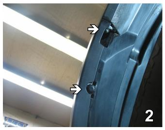
Just forward of the front tire, inside the wheel well, remove pushpin and Phillips screw. Do this to both sides of the vehicle. Set push pins and screws aside to reinstall later.
