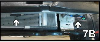
7. Disconnect wire connections from the right and left side of the bumper, as well as the sensors located underneath the bumper.
