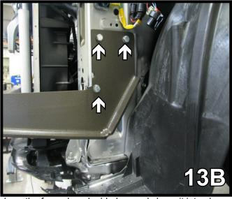
13. Take the baseplate and slide it up to the very top edge of where the frame has doubled up and clamp it into place. When positioned in place, drill three holes using a 13/32" drill bit. Then insert a 3/8-16x1 1/2" hex bolt with a 3/8" lock washer into those holes and tighten to nut plates. Cut the excess nut plate wire so that it is flush with the frame rail. Do this to both sides of the vehicle.
