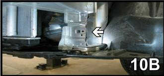
10. Using a marker, make a horizontal line just below the metal bumper. Then with a reciprocating saw, cut into the edge of the frame well and follow it down to the bottom and out. It's very important to follow the frame well because it offsets down at the top. You will then be able to remove that whole portion of the frame well webbing. Do this to both sides of the vehicle.
