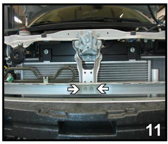
11. Using a 10MM socket, remove two metric bolts from the center of the bumper. Carefully remove bumper and set aside with bolts to be reinstalled later.
