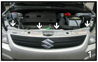
Remove four metric bolts with a 10MM socket or a Phillips screw driver. Set bolts aside to be reinstalled later.
