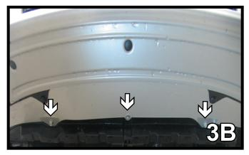
Just forward of the front tire, on the bottom side of the fascia, remove three Phillips screws from both sides of the vehicle. Then remove one Phillips screw and two metric bolts from the center of the fascia using a 10MM socket or Phillips screw driver. Set screws and bolts aside to reinstall later.
