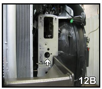
12. Using a 1 1/4" hole saw, drill a hole just to the off side of the threaded hole so you can get into the lower portion of the frame to position a nut plate. Do this to both sides of the vehicle.
