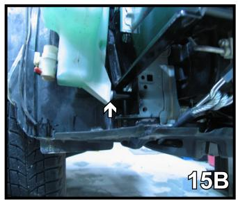
15. Reinstall the washer reservoir using 6MM -1.0 x 30MM hex bolts, 14" flat washers and 1 1/2" pipes in the two top holes. In the bottom hole, use a 6MM-1MM X 80MM hex bolt, 1/4" flat washer and 2 1/2" tube.
