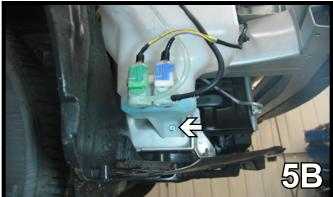
Using a 10MM socket, remove two metric bolts on top and one metric bolt on the bottom. You will then need to plug the hoses and disconnect the electrical. Set washer reservoir aside to reinstall later.
