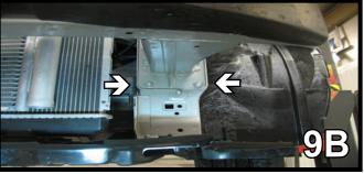
Using a 12MM socket, remove two metric bolts from the top and bottom of the bumper. Do this to both sides of the vehicle. Set bolts aside to be installed later.
