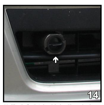
14. Align the fascia to its original position and, using a hack saw knife, trim if necessary the opening in the grille for the attachment tabs. Do this to both sides of the vehicle. When using power drills be aware of the dangers of torque and drill bit length.
