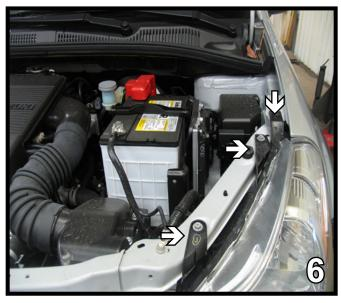
6. Using a 10MM socket, remove two metric bolts on top and one metric bolt on the bottom of the headlight assembly. There is also a pushpin in the same area as the top bolts that needs to be removed. Pull the headlight assembly forward to remove and disconnect the electrical connections. Do this to both sides of the vehicle. Set bolts, pushpin and headlight assembly aside to reinstall later.
