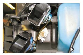
Using the 10MM socket, remove metric bolt from horn bracket on the driver's side and set assembly aside.
