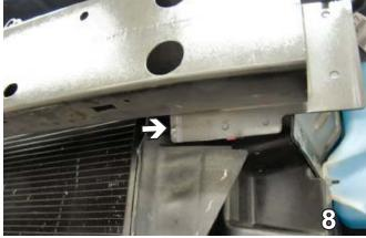
8. Tap and bend the inside portion of frame end plate toward radiator 1/4" with the hammer, both sides.
