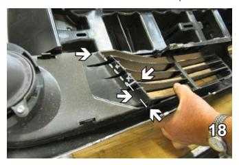
18. Lay fascia face down on a soft surface, so as not to scratch, using the utility knife, cut and remove 1/2" of the outer edge of fascia's opening, both sides.
