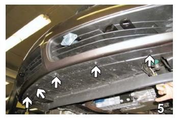
Remove the five metric bolts from lower edge of fascia with the 7MM socket, pull corners of fascia to the side of vehicle to release tabs, pull fascia forward and set aside.
