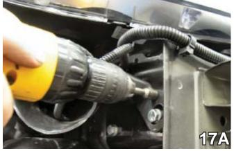
17. Remove rubber grommet from the front bolt location on the air baffle. Reinstall the air baffle on the passenger's side to its original position, using the existing metric bolt and lower push pin. Slide front bolt location over the top of front bolt of baseplate. Using the 5/16" nut driver and drill, install the #10 x 1 self drilling screw through air baffle webbing and into frame. This will help to stabilize the air baffle. Do not drill into baseplate.
