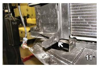
11. Remove one christmas tree push pin from lower air dam, just below metal bumper, both sides. Turn air dam in to lay flat against radiator and lift up to remove, both sides.
