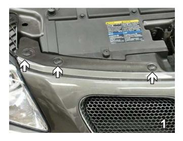
1. Remove the six push pins from the top edge of fascia just between headlight assemblies.
