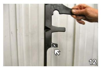
Using the utility knife, cut and remove the small tab of air dam and reinstall both sides. This will open area just below metal bumper for baseplate install.
