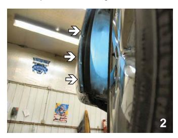
Remove two christmas tree push pins and one metric bolt from the edge of wheel well, just forward of front tire with the 7MM socket, both sides.
