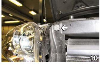
Remove one christmas tree push pin from upper air dam, just inside headlight assembly, both sides.
