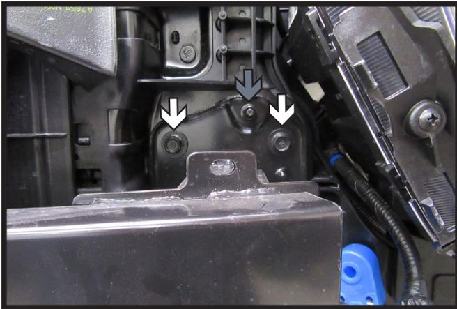
6. Using a 12MM socket, remove the four (4) bolts (white) from the bumper. Then using a 10MM socket, remove the one (1) bolt (gray) from the bumper. This bolt is above the bumper on the driver side and below the bottom of the bumper on the passenger side. Do this on both sides of the vehicle. Remove bumper and set aside, it will not be reinstalled.
