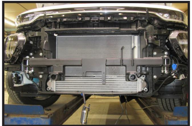
13. Start the remaining four (4) bolts, two (2) on each side to the front of the baseplate. Set the cross tube onto the side brackets. Place the four (4) 1/2" bolts with flat washer and lock washer into holes. Do not add hardware to the bottom of bolts.
