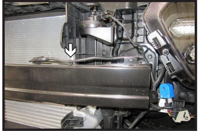
5. Unclip the temperature sensor wire loom from the bumper on the driver side of the vehicle. Let hang to be reinstalled later.
