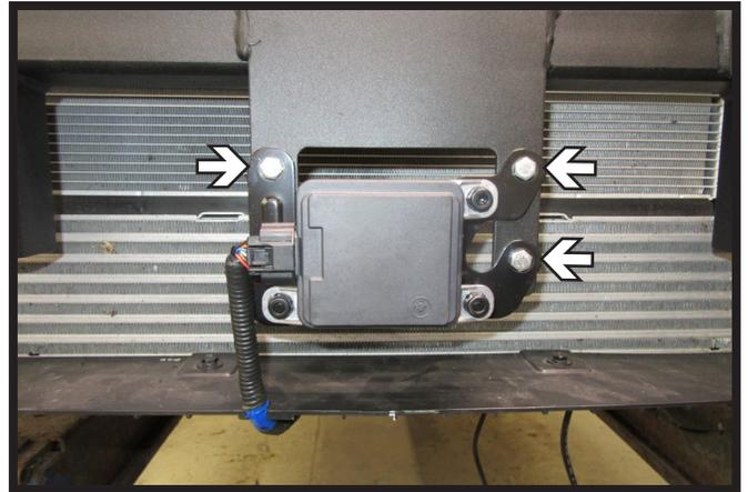
15. Attach the ACC to the bracket on the baseplate using three (3) 1/4" x 3/4" bolts with nylon lock nut.
