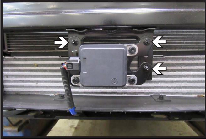
4. Using a 10MM socket, remove the three (3) bolts from the Adaptive Cruise Control (ACC) bracket. Let ACC hang to be reinstalled later.
