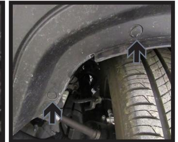
7. Using a 10MM socket, remove the seven (7) bolts (white) from the belly pan. There are four (4) in the front and three (3) in the back. Use your fingers or a 14MM socket to remove the one (1) plastic bolt (gray) from the belly pan. Then remove the four (4) push pins (black), two (2) from each side. Remove belly pan and set aside to be reinstalled later.
