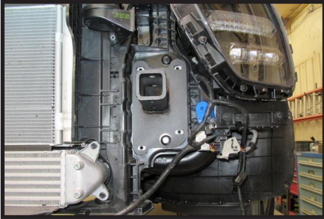
10. Slide the baseplate into the frame with the hole towards the radiator. Do this on both sides of the vehicle.
