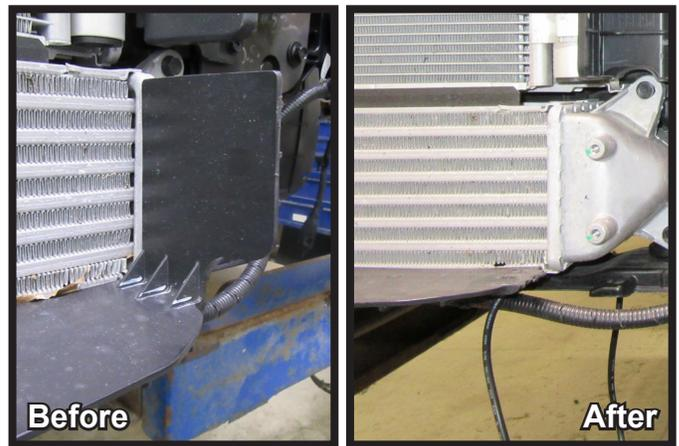
9. Using a reciprocating saw, trim the shroud on each side so that the bottom is flush and the sides are removed as shown.
