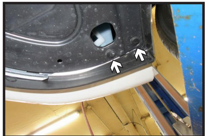
3. Remove the eight (8) push pins from the underside of the fascia. There are four (4) on each side. Remove fascia by lifting and pulling, starting on the side, to release clips along each side as well as the center. Set fascia aside to be reinstalled later.
