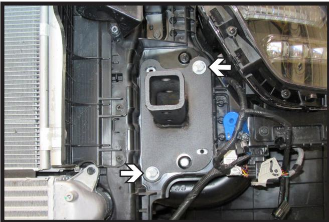
12. Start the two (2) 8MM bolts with hardware as shown. Do this on both sides of the vehicle. Leave loose at this time.
