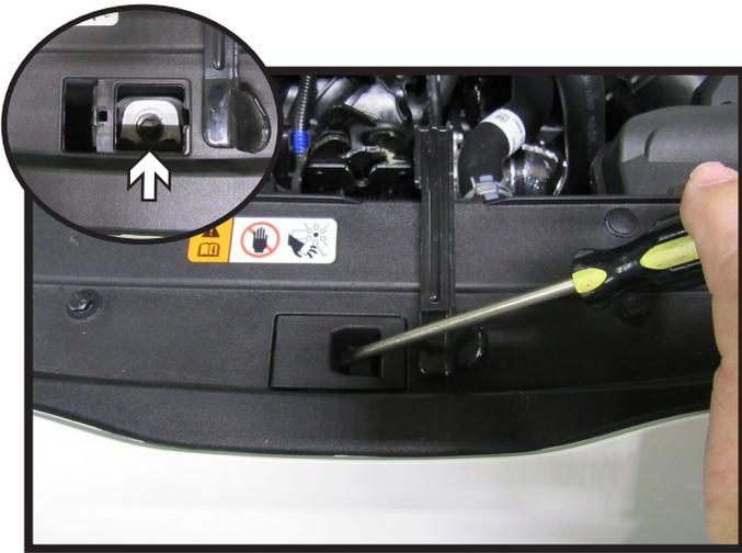
1. Using a flat screw driver, pop out the plastic piece in the middle of the fascia cover. Using a 10MM socket, remove the one (1) bolt (inset)
