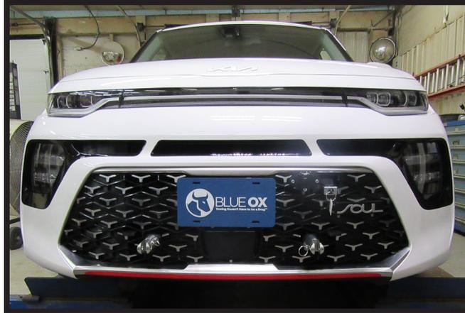
18. Hold the fascia as close to its original position, mark and trim the fascia around the convenience links and attachment tabs. Reinstall the belly pan and fascia.
