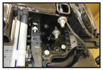
15. Attach the permanent baseplate safety cables to the provided convenience link on the baseplate. The photo above shows the recommended installation of the cables to frame of vehicle. Additional options may interfere with suggested mounting; in this case, secure the cables to a solid piece of the frame as described in the General Information sheet. Be sure the safety cables do not rub against any hoses or moving parts. Do this on **BOTH** sides of the vehicle.
