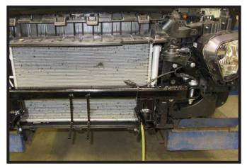
13. Using the provided zip ties attach the temperature sensor loom to the baseplate on the driver side of the vehicle as shown.
