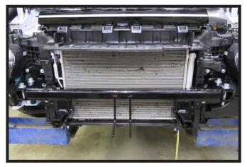
Start the remaining four (4) bolts, two (2) on each side to the front of the baseplate. Set the cross tube onto the side brackets. Place the four (4) 1/2" bolts with flat washer and lock washer into holes. Do not add hardware to the bottom of bolts.
