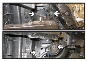
5. Using a 13MM socket, remove the four (4) bolts (white) from the bumper. Then using a 10MM socket, remove the two (2) bolts (gray) from the bumper. Do this on both sides of the vehicle. Remove bumper and set aside, it will not be reinstalled later.
