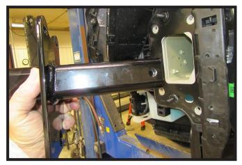
8. Slide the baseplate into the frame with the hole towards the radiator. Do this on both sides of the vehicle.
