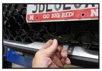
14. **Optional Breakaway:** Attach breakaway bracket to the electrical rods and trim fascia as needed.
