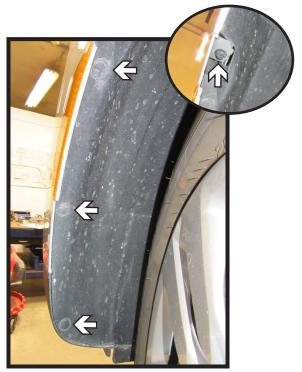
Remove the three (3) push pins from along the edge of the wheel well. Using a 10MM socket remove the one bolt (inset). Do this on both sides of the vehicle.
