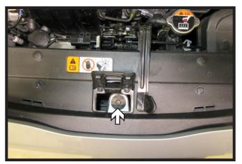
1. Lift the cover next to the handle on top of the fascia. Using a 10MM socket, remove the one (1) bolt.
