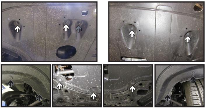
Using a 10MM socket, remove the seven (7) bolts (white) from the belly pan. There are four (4) in the front and three (3) in the back. Using a 14MM socket, remove the one (1) plastic bolt (gray) from the belly pan. Then remove the four (4) push pins (black), two (2) from each side. Remove belly pan and set aside to be reinstalled later.
