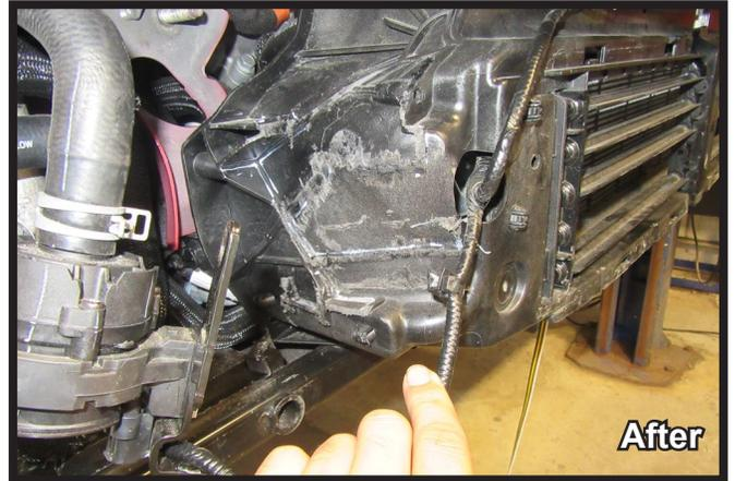
15. Using a reciprocating saw, shave the ribs on the passenger side of the vehicle as shown so they are flush with the shutter housing to allow clearance for the baseplate.
