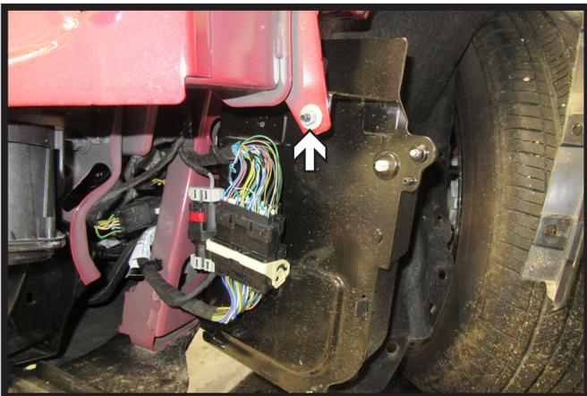
11. Using a 10MM socket, remove the one (1) bolt from the top of the black box in front of the wheel on the driver side of the vehicle (left). Then remove the wire loom from the backside bottom bolt. Using a 10MM deep socket, remove the two (2) bolts from the backside (right). Let box hang out of the way for baseplate installation.
