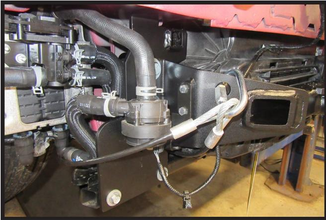
34. Attach the permanent baseplate safety cables to the provided convenience link on the baseplate. The photo above shows the recommended installation of the cables to frame of vehicle. Additional options may interfere with suggested mounting; in this case, secure the cables to a solid piece of the frame as described in the General Information sheet. Be sure the safety cables do not rub against any hoses or moving parts. Do this on **BOTH** sides of the vehicle.
