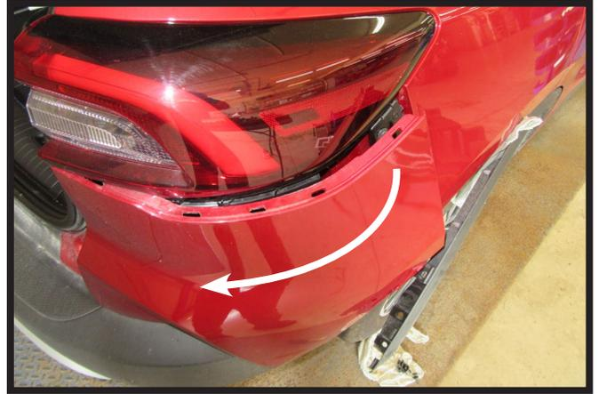
4. Remove the rear panel below the tail light housing. Do this on both sides of the vehicle.
