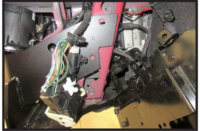
25. Remove the four (4) push pins attaching the electrical bracket and loom to the black box on the driver side of the vehicle.
