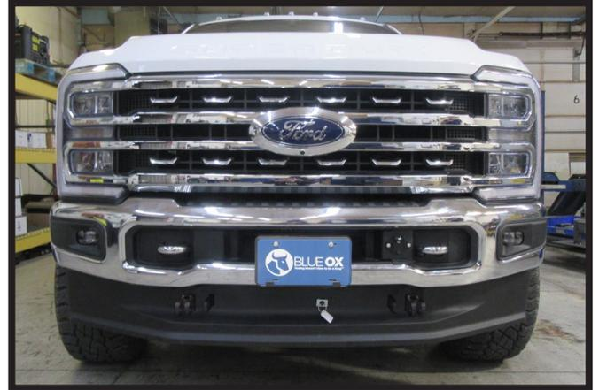
5. Attach the permanent baseplate safety cables to the provided convenience link on the baseplate. The photo above shows the recommended installation of the cables to frame of vehicle. Additional options may interfere with suggested mounting; in this case, secure the cables to a solid piece of the frame as described in the General Information sheet. Be sure the safety cables do not rub against any hoses or moving parts. Do this on **BOTH** sides of the vehicle.
