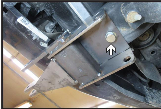
3. Install the 5/8" x 1-3/4" bolt with lock washer into bottom hole of the baseplate. Insert 5/8" wire nut between the top of the baseplate and bumper. Do this on both sides of the vehicle. Tighten bottom bolt then tighten side bolts.
