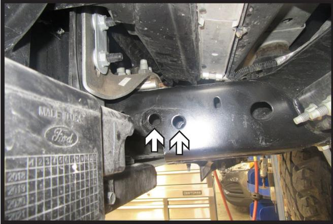
1. Before installing the baseplate, ensure the 5/8" x 6-1/2" bolts will go completely through the frame. Holes may not fully line up on each side of the frame. If not ream out holes as needed.
