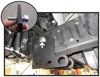
Attach outer side plate using 3/8" bolt with lock washer, flat washers and nut plate. Leave loose. Do this on both sides of the vehicle.
