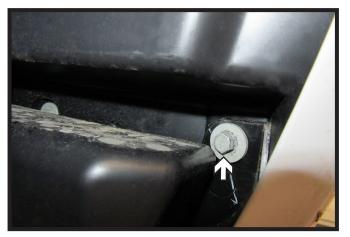
5. For Vehicles with a Shroud: Using a 10MM socket, remove the one (1) bolt from in front of the tire. Do this on both sides of the vehicle. Remove plastic shroud and set aside to be reinstalled later.
