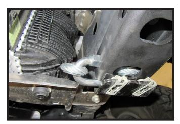
6a. Raptor Models: Attach the permanent baseplate safety cables to the provided convenience link on the baseplate. The photo above shows the recommended installation of the cables to frame of vehicle. Additional options may interfere with suggested mounting; in this case, secure the cables to a solid piece of the frame as described in the General Information sheet. Be sure the safety cables do not rub against any hoses or moving parts. Do this on BOTH sides of the vehicle.
