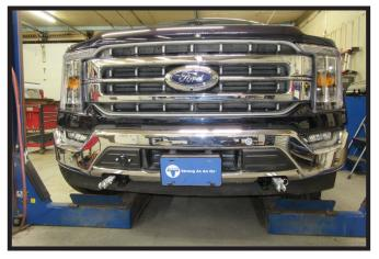
8a. Standard Models: Reinstall the bumper and reconnect all electrical connections.
