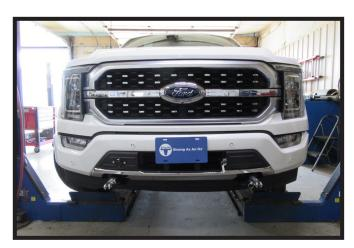
8b. **Hybrid Models:** Reinstall the bumper, fascia, fascia cover and reconnect all electrical connections.
