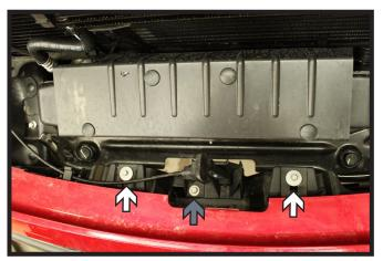
3. Unclip the cable from the clamp on the passenger side (left). Using a 8MM socket, remove the two (2) bolts from the middle of the bumper (right-white). Then using a 10MM socket, remove the center bolt from the middle of the bumper (right-gray). Remove the bumper from the vehicle disconnecting any electrical connections and set aside.
