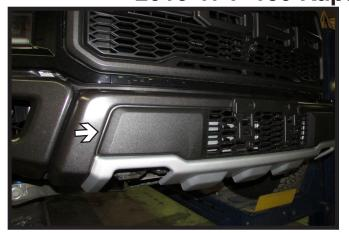
Unsnap the plastic cover from the face of 1. the bumper. Do this on both sides of the vehicle.
