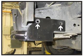
Using a 17/32" drill bit, drill the existing holes thru the frame. Install 1/2"-13 x 1-3/4" bolts with lock washers into the holes with 1/2"-13 nut plates on the inside of the frame. Do this on both sides of the vehicle. Fully tighten all hardware.
