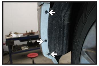
Using a 7MM socket, remove the three (3) screws from the edge of the wheel well. Do this on both sides of the vehicle.
