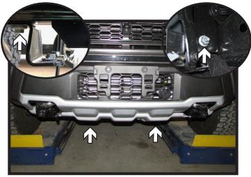
Using a 15MM socket remove the six (6) 3. bolts holding the skid plate. Then using a 15MM socket remove the one (1) bolt from the skid plate bracket on each side of the vehicle (left inset).
