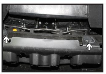
4. On the underside of the fascia towards the middle, remove the two (2) push pins.
