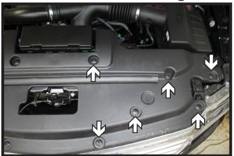
Using a Phillips screwdriver, remove the twelve (12) push pins from the top edge of the fascia cover. There are six (6) on each side. Set the cover aside.
