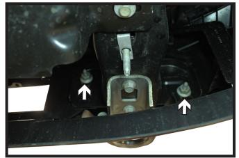
2. Using a 21MM socket, remove the two (2) nuts from the backside of the bumper. Do this on both sides of the vehicle.
