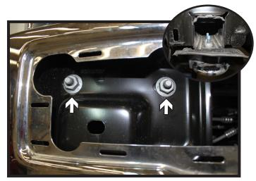
4. Using a 21MM socket, remove the two (2) nuts from the face of the bumper. Do this on both sides of the vehicle.
