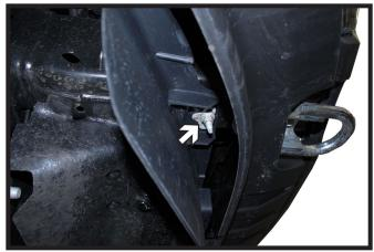
1. Using a 15MM socket, remove the nut in front of the lower valance. Do this on both sides of the vehicle.
