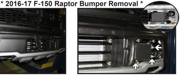
2. If equipped with Adaptive Cruise, using a 11MM socket, remove the three (3) nuts from the ACC sensor. Unsnap the sensor. disconnect the electrical connection and set aside.
