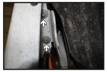
Using a 10MM socket, remove the two (2) screws from inside edge of the fascia/ fender joint. Do this on both sides of the vehicle.
