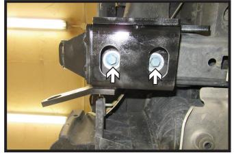
Install the baseplate to the frame with the existing hardware. Do this on both sides of the vehicle. Fully tighten all fasteners. (Note: If tow hooks are not present, use the supplied hardware for baseplate installation.) (Note: Ensure that the outer side plate is tight against the frame.)
