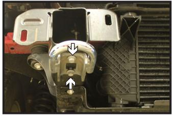
Using a 15MM socket, remove the two (2) bolts from the tow hook. Do this on both sides of the vehicle. Do not discard the existing hardware.
