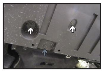
6. Using a 7MM socket, remove the two (2) bolts (white) and one (1) push pin (gray) from the belly pan. Do this on both sides of the vehicle.
