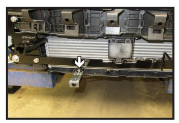
24. **Optional Breakaway**: Using the provided 1/4" hardware, attach the breakaway switch to the bracket on the baseplate as shown.
