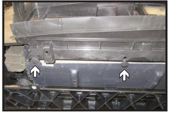
Remove the four (4) push pins from along the underside of the shutter housing.
