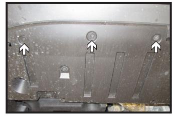
5. Using a 5.5MM socket, remove the twelve (12) bolts from the belly pan. There are six (6) on each side.
