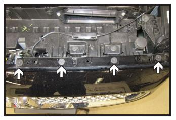
2. Using a T20 Torx, remove the seven (7) screws from the top of the fascia. There are four (4) on the driver side and three (3) on the passenger side.
