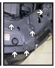
1. Remove the sixteen (16) push pins from the fascia cover. Set cover aside to be reinstalled later.
