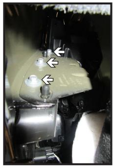
4. Pull back the wheel well liner. Using an 8MM socket, remove the three (3) bolts from the wheel well joint. Do this on both sides of the vehicle.
