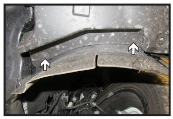
7. Using a 5.5MM socket, remove the two (2) bolts from in front of the tire on the underside of the vehicle. Do this on both sides of the vehicle. Remove belly pan and set aside to be reinstalled later.
