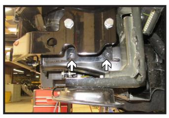
20. Using a 3/8" drill bit, drill out the bottom two (2) holes using the holes on the side plate as a guide. Install the provided 3/8" hardware. Do this on both sides of the vehicle.
