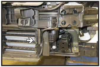
9. Unsnap the temperature sensor wire loom and place out of the way. It will be remounted later.
