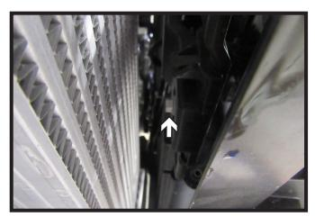
12. Using a 7MM socket, on the backside of the shutters, remove the one (1) bolt from the shutter housing.
