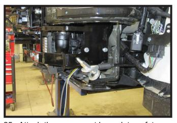
25. Attach the permanent baseplate safety cables to the provided convenience link on the baseplate. The photo above shows the recommended installation of the cables to frame of vehicle. Additional options may interfere with suggested mounting; in this case, secure the cables to a solid piece of the frame as described in the General Information sheet. Be sure the safety cables do not rub against any hoses or moving parts. Do this on **BOTH** sides of the vehicle.
