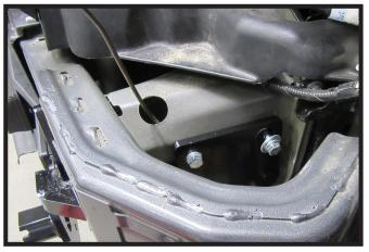
17. Line up the side plate and tart the top two (2) 3/8" bolts but leave loose at this time. Use a 3/8" bolt with lock washer for the front hole. Use a 3/8" bolt with a flat washer and lock washer for the back bolt. Do this on both sides of the vehicle
