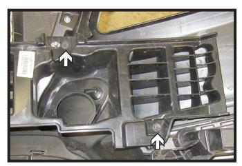
26. Using a 7MM socket remove the four (4) bolts, two (2) on each side, holding the plastic piece to the back of the fascia.
