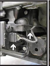
11. On the driver side of the vehicle unplug the electrical cable for the ACC sensor and remove the pin holding the electrical cable to the frame. Reroute the cable behind frame bracket and reattach pin and plug back into the ACC sensor.
