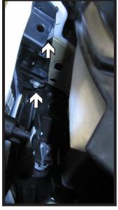
3. Using a 7MM socket, remove the three (3) bolts in front of the tire on the wheel well (white, left). Using a Phillips screwdriver, remove the one (1) screw (gray). Remove the one (1) push pin (black). Pull the wheel well cover back. Using an 8MM socket, remove the two (2) bolts (white, right). Do this for both sides of the vehicle.
