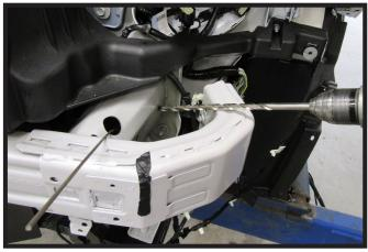
15. Using a 3/8" drill bit, ream out the rear existing hole. Do this on both sides of the vehicle.
