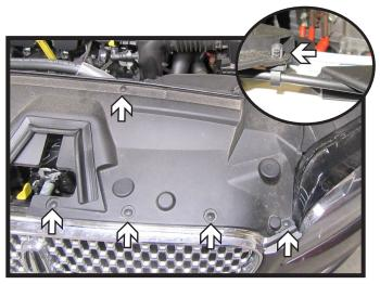
1. Remove the ten (10) push pins from the fascia cover. There are five (5) on each side. On the driver side, remove one (1) push pin and unhook the cover. Set the cover aside.
