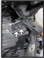
6. Using a T25 Torx, remove the one (1) screw from the plastic headlight cover (white, left). Remove the two (2) push pins (black). Pull the plastic cover up. Using a 10MM socket, remove the two (2) exposed bolts (white, right). Do this for both sides of the vehicle.
