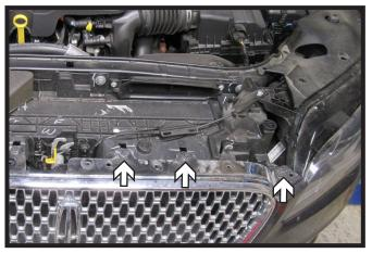
2. Using a 10MM socket, remove the six (6) bolts from the top of the grill cover. There are three (3) on each side.
