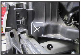
21. Remove the indicated area to allow for bracket to fit behind frame. Do this on both sides of the vehicle.
