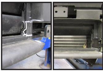
13. Then trim indicated area from on the shutter housing and remove the bottom shutter. Do this on both sides of the vehicle.
