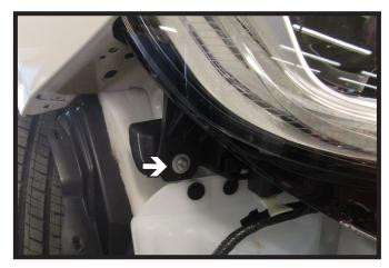
7. Using a T30 Torx, remove the three (3) bolts from the headlight. Do this for both sides of the vehicle.
