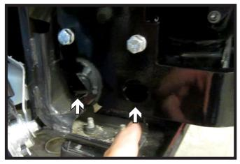
19. Using a 3/8" drill bit, drill the lower plate holes through the support. Do this on both sides of the vehicle. Fully tighten all hardware.
