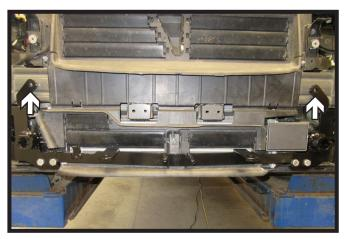
20. Using a 1/2" drill bit, drill out the top two(2) holes as indicated.
