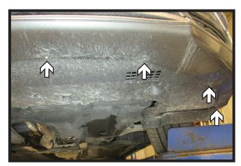
4. Using a 7MM socket, remove the eight (8) bolts from the underside of the fascia. There are four (4) bolts on each side.
