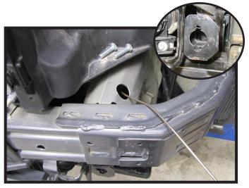
14. Using a 1-1/4" hole saw, drill access holes in the side of the frame as shown and in the face of the lower support (inset). Do this on both sides of the vehicle.
