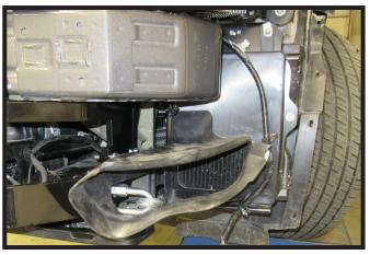
25. Reattach air bathel to the driver side of the vehicle. Air bathel may need to be trimmed to allow it to fit around safety cables and onto the vehicle properly.
