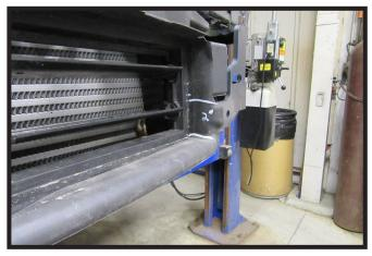
12. Measure 2" up form the bottom of the shutter housing and trim the indicated are. Do this on both sides of the vehicle.
