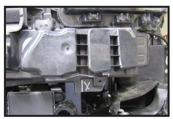
27. Hold the plastic piece and mark as shown the areas that interfere with the baseplate. Then trim indicated areas to allow to fit around baseplate. After trimmed reinstall plastic piece to the back of the fascia.
