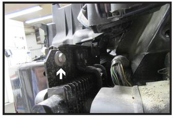
Using a 10MM socket remove the bolt holding the air bathel on the driver side of the vehicle and remove to be reinstalled later.
