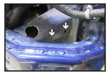
Using a 3/8" drill bit, ream out the rear existing hole. Do this on both sides of the vehicle.
