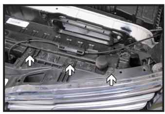
3. Using a 10MM socket remove the three (3) bolts from the top of the fascia. Do this on both side of the vehicle.
