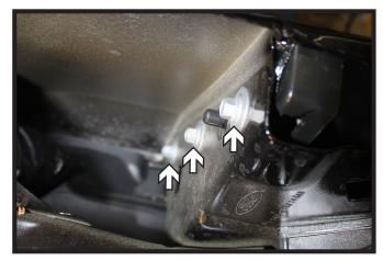
5. Using a 8MM socket, remove the three (3) bolts from the fascia/fender joint underneath where the headlight was. Do this on both sides of the vehicle.
