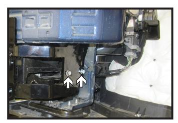
16. Using two (2) 3/8" bolts attach the Z bracket to the side plate as indicated.
