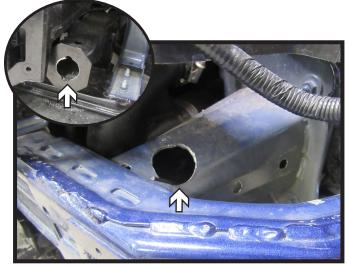
13. Using a 1-1/4" hole saw, drill access holes in the side of the frame as shown and in the face of the lower support (inset). Do this on both sides of the vehicle.
