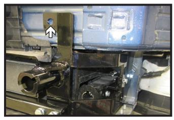
18. Using a 1/2" drill bit drill out top two (2) holes, one (1) on each side. Metal is extremely hard so may need to start with a 1/4" drill bit then work up to a 3/8" drill bit and then eventually use a 1/2" drill bit to create the holes. Make sure to drill slowly.
