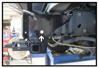
4. Position the baseplate onto the frame flush with the top of the frame rail and as far forward as possible (gray). Level and clamp the baseplate securely. Using a 1/2" drill bit, drill one (1) hole thru the frame on each frame rail. Install a 1/2"-13 x 1-1/2" bolts with a 1/2" lock washers into the holes and secure with 1/2" nut plates on the inside of the frame. Fully tighten both fasteners.
