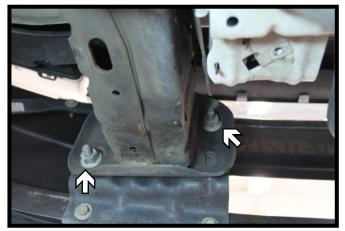
3. Using a 21MM socket, remove the four (4) nuts from the inside of the bumper. There are two (2) on each side. Set the bumper aside.
