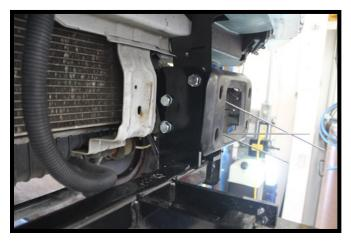
Using a 1/2" drill bit, drill the inside holes thru the frame on each frame rail. Install a 1/2"-13 x 1-1/2" bolts with a 1/2" lock washers into the holes and secure with 1/2" nut plates on the inside of the frame. Fully tighten all fasteners.
