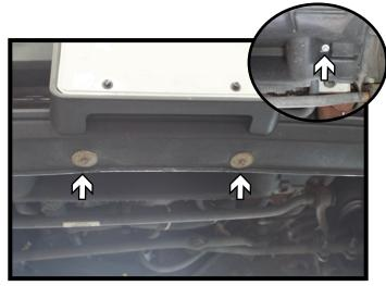
Using a 8MM socket, remove the four (4) screws from the bellypan. There are two (2) in front and one (1) on each back corner. The bellypan will not be reinstalled.
