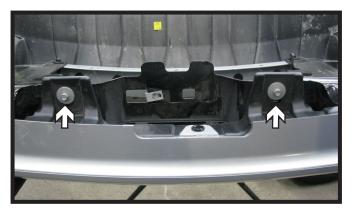
Using a 8MM socket, remove the two (2) bolts from the top side of the bumper. Unhook any electrical connections and pull the bumper from the vehicle.
