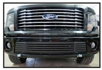
11. Harley Edition Only: Hold the bumper as close to it's original position. Mark the bumper for cutting out around the baseplate. Using a utility knife, trim the bumper and reinstall.
