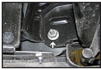
From the underside of the bumper, using a 21MM socket, remove the bolt from the outer side of the frame. Do this on both sides of the vehicle.
