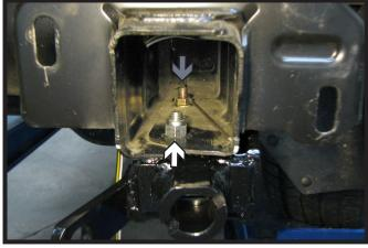
7. The front bolt (white) uses a 1/2"-13 nylon hex nut. The back bolt (gray) uses a 1/2"-13 whiz nut plate. Tighten down while pushing the plate toward the frame. Do this to both sides.
