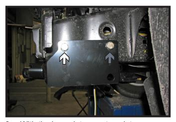
8. With the baseplate as a template, use a 17/32" drill bit to drill the two (2) holes on the sides of the baseplate. Insert a 1/2"-13 x 1-3/4" hex bolt, 1/2" lock washer and 1/2"-13 nylon hex nut into the front hole (white). Then insert a 1/2"-13 x 1-3/4" bolt, 1/2" lock washer and 1/2"-13 whiz nut plate into the back hole (gray).
