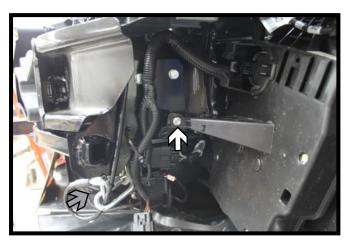
19. Bend the webbing bracket back to its original position and reinstall the 10MM bolt (white).
