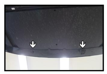
3. On the underside of the fascia, using a flat screwdriver, remove the two (2) pushpins from the front outer edge.
