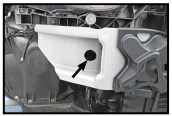
10. On the front bumper, using a 1-1/4" hole saw, slowly drill a hole centered vertically and horizontally on the flat area as shown. Do this on both sides of the vehicle. NOTE: The hole cut is used to place nut plates for future steps.
