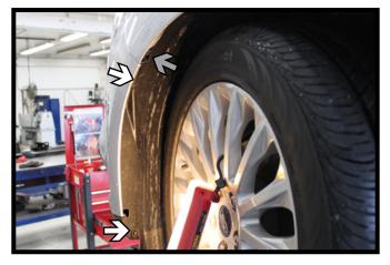
Using a T27 Torx, remove the two (2) screws from the driver's side front wheel well (white arrows). Using a flat screwdriver, remove the push pin from the driver's side front wheel well (gray arrow). Repeat this on the passenger's side.
