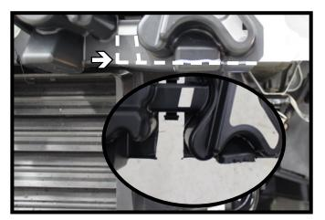
12. On the plastic bumper cover, using a utility knife, trim the lower outer edge flush with the bottom of the bumper, also trim the vertical space between the protrusions as shown for the clearance of the baseplate tabs. Repeat on the other side of the vehicle.
