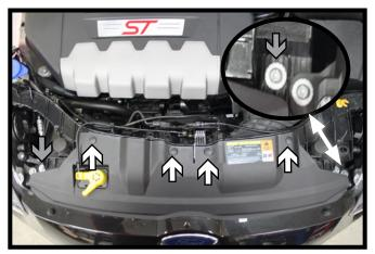
From the top of the fascia, using a T30 Torx, remove the inner-most bolt from each side (gray arrow). Using a flat screwdriver, remove the four (4) push pins (white arrows).
