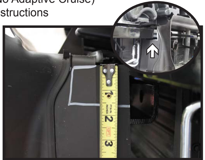
21. To reattach the intake cover, use a utility knife to cut from the back upper corner of the side wall a 2 1/2" x 1 1/2" rectangle from each side of the cover. Reinstall using the two (2) T30 Torx bolts. NOTE: If a breakaway will be installed, install the breakaway before installing cover. Be sure that bottom of the cover goes below the breakaway bracket.
