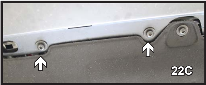
22. Optional: To install a breakaway switch, you must remove the belly pan with a T30 Torx. Remove the two (2) screws from in front of both the driver's and passenger's side tires (22A) then follow the pan toward the middle of the vehicle removing the three (3) specified bolts (22B and 22C).
