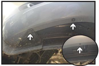
4. **2014 Models:** Using a 7MM socket, remove the five (5) screws from the underside of the fascia. There are two (2) in each corner and one (1) in the middle.
