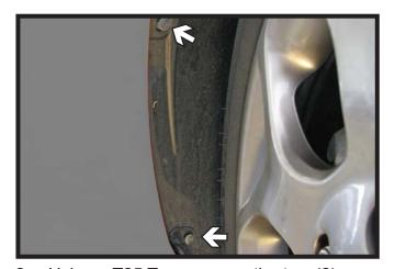
2. Using a T25 Torx, remove the two (2) screws from the wheel well. Do this on both sides of the vehicle.
