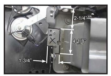
Using a reciprocating saw, trim the face of the frame as shown for baseplate clearance. Do this on both sides of the vehicle.
