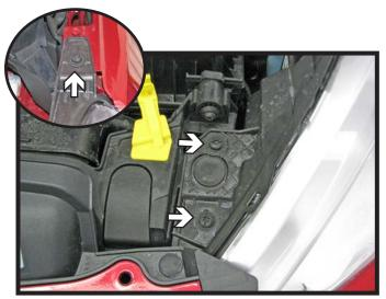
5. **2011-13 Models:** Using a T30 Torx, remove the three (3) screws from the headlight. Disconnect the electrical line and set the head light aside. Do this on both sides of the vehicle.
