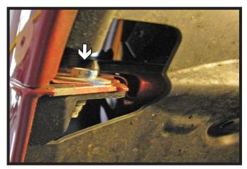
3. Using a 8MM socket, remove the screw from the upper edge of the wheel well. Do this on both sides of the vehicle.
