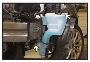
7. Disconnect the wire loom clips from the frame (gray). Using a 10MM socket, remove the two (2) screws from the washer fluid reservoir (white). Disconnect all lines and plug fluid lines. Set the reservoir aside.
