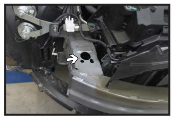
9. Using a 1-1/4" hole saw, drill an access hole on top of the bumper as shown. Do this on both sides of the vehicle.
