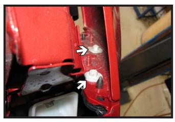
6. Using a 8MM socket, remove the two (2) screws from the edge of the fascia underneath the headlight. Do this on both sides vehicle.
