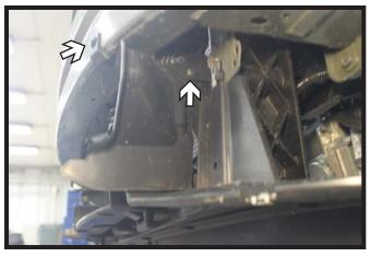
11. **2014 Models:** Using a Phillips screwdriver, remove the two (2) screws from the plastic shroud. Do this on both sides of the vehicle.
