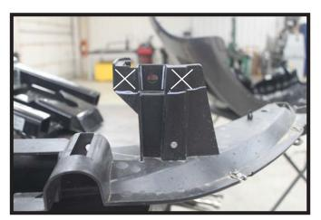
2014 Models: Remove the two (2) screws from the plastic shroud and trim the outer portions for baseplate clearance. Do this on both sides of the shroud and reinstall.
