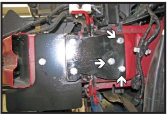
15. Using a 13/32" drill bit, drill the three (3) holes thru the frame. Install 3/8"-16 x 2" bolts with 3/8" lock washers into the holes and 3/8"-16 nut plates on the inside of the frame. Do this on both sides of the vehicle. Fully tighten all fasteners.
