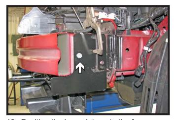
13. Position the baseplate onto the frame, flushing the top of the baseplate and the frame. Push the baseplate back as far as possible, level and clamp into position.
