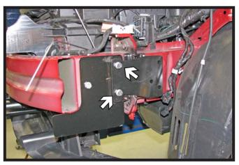
14. Using a 13/32" drill bit, drill the remaining two (2) holes thru the frame. Position the correct support plate for each side and be sure it is level with the frame. Install 3/8"-16 x 2" bolts with 3/8" lock washers into the holes and 3/8"-16 nut plates on the inside of the frame. Do this on both sides of the vehicle. Fully tighten all fasteners.
