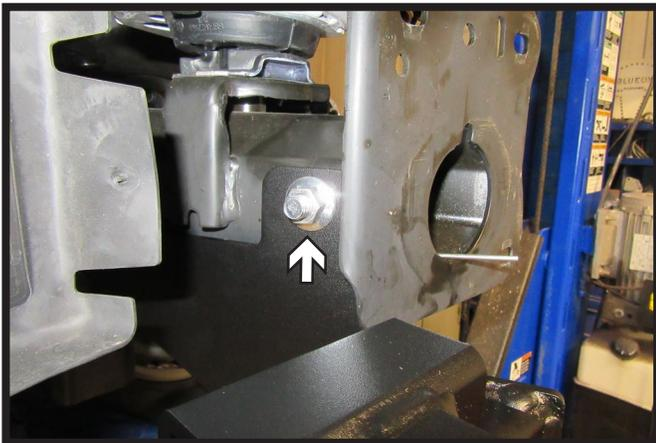
20. Start the one (1) 1/2" carriage bolt with plate and whiz lock nut in side hole of the baseplate. Tighten bottom bolt then side bolt. Do this on both sides of the vehicle.
