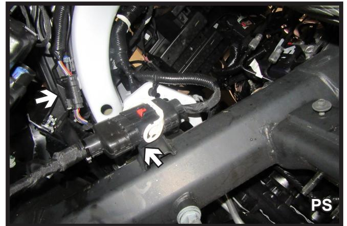
10. Unplug the three (3) electrical connections, one (1) on the driver side and two (2) on the passenger side, from behind the bumper.
