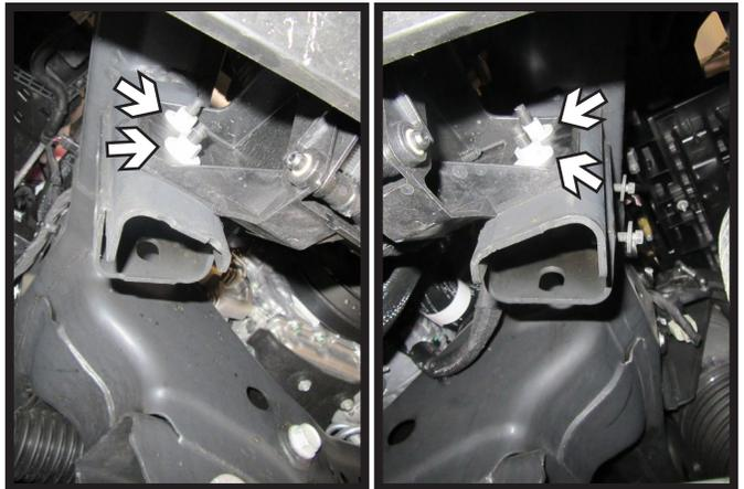
7. Using a 13MM socket, remove the four (4) nuts, two (2) on each side. Remove valence and set aside to be reinstalled later.
