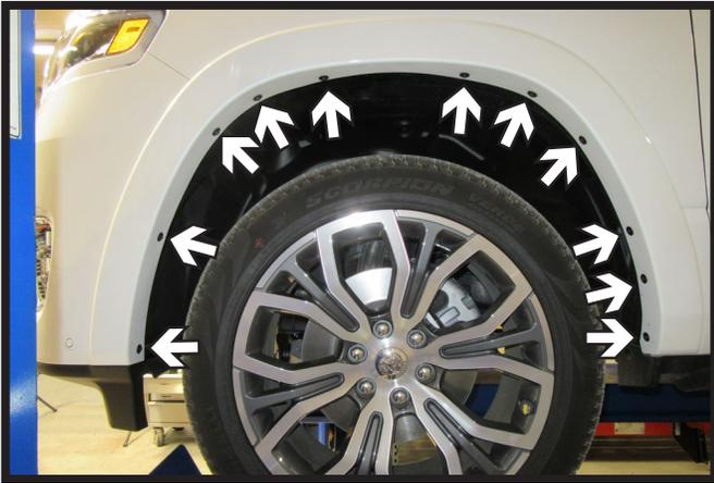
1. Using an 8MM socket, remove the eleven (11) bolts from the wheel well trim. Do this on both sides of the vehicle.
