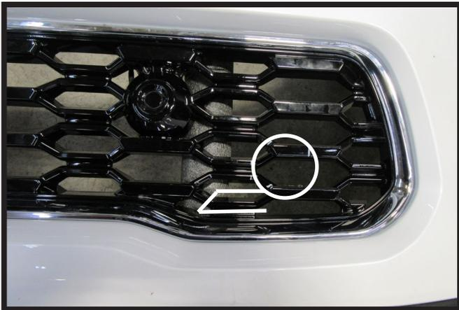
28. Hold the fascia as close to its original position, mark and trim the fascia around the convenience links and attachment tabs. Example shown above.
