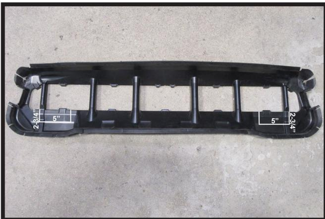
24. Using a reciprocating saw remove the indicated area of the shutter housing to allow clearance for the baseplate and convenience links. Measure 2-3/4" down on the outside of the outer rib. Then measure 5" towards the center of the housing. Finally measure 2-3/4" up from the 5" line to the center opening. Remove area. Do this on both sides of the shutter housing.
