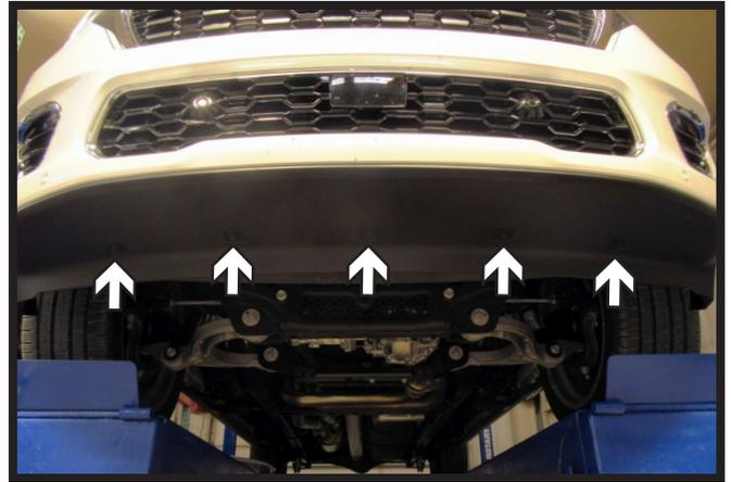
5. Using a 10MM socket, remove the five (5) bolts from the bottom of the fascia.
