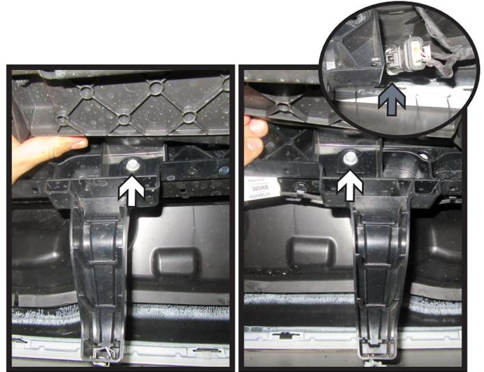
9. Using a 10MM socket, remove the two (2) bolts from the plastic piece behind the bumper. Remove the electrical clip from each end of the plastic piece (inset). Remove piece and set aside to be reinstalled later.
