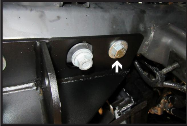
22. Install one (1) 1/2" bolt with flat washer and whiz nut in the back bottom hole of the baseplate. Tighten. Do this on both sides of the vehicle.
