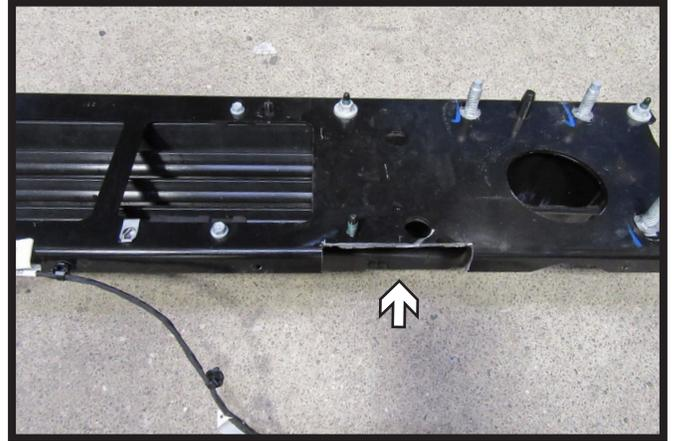
15. Using a reciprocating saw remove the marked area as shown. Be careful not to cut the wire loom attached to the bumper. Do this on both sides of the bumper.
