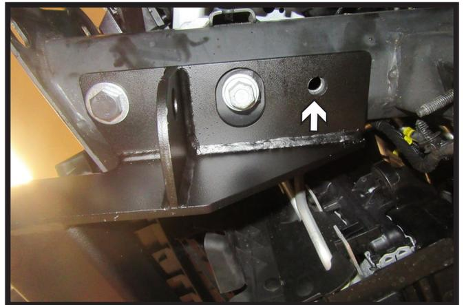
21. Using a 1/2" drill bit, drill out the back bottom hole using the baseplate as a template. Do this on both sides of the vehicle.
