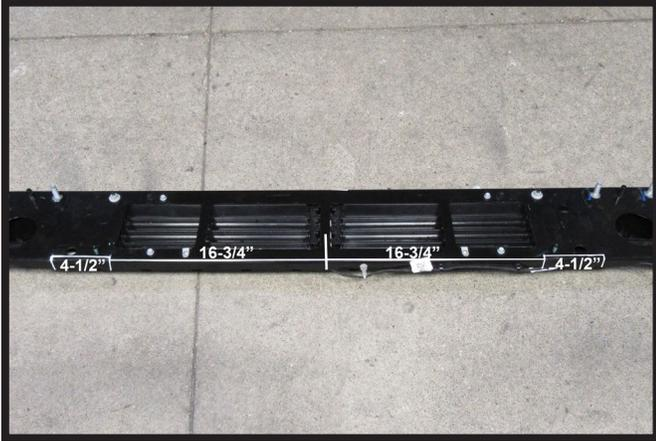
14. Mark the center point on the back of the bumper. Measure 16-3/4" in each direction and mark. Then measure 4-1/2" and mark again.
