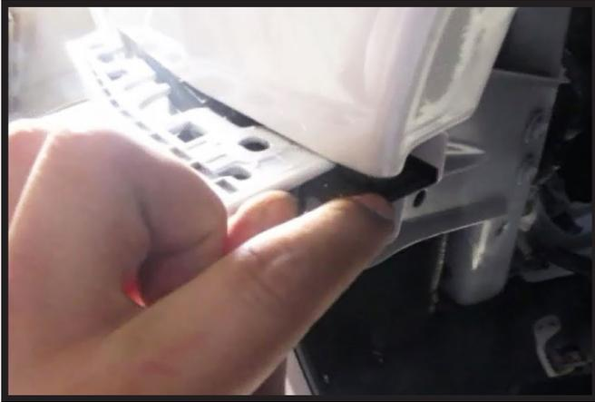
11. Start to remove the fascia at the fascia joint. To release the fascia, push up on the fascia and down on the black piece behind. Do this on both sides of the vehicle. Remove fascia and set aside to be reinstalled later.
