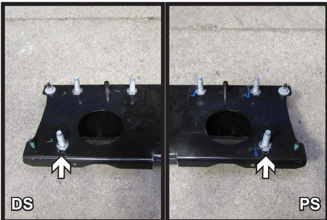
16. Remove coil piece from the bottom bolt on each side. Remove the two (2) bolts from the bumper.
