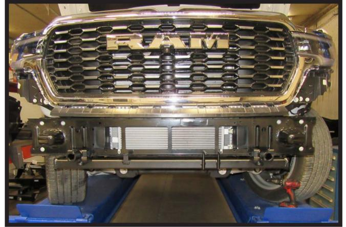
23. Reinstall the bumper piece onto the vehicle.
