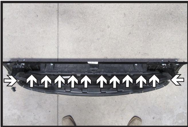
13. Remove the shutter housing from the shutters by unclipping the ten (10) clips on the top, ten (10) on the bottom and one (1) on each side. Remove shutter housing and set aside to be reinstalled later.
