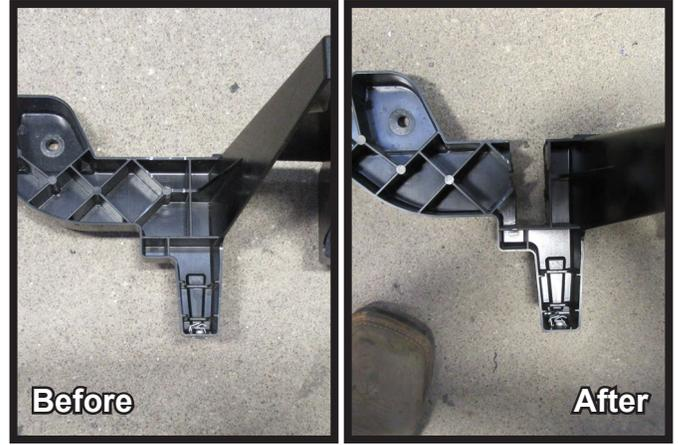
27. Using a reciprocating saw, trim the plastic piece from behind the bumper as shown. Do this on both sides of the piece. Reinstall plastic piece.
