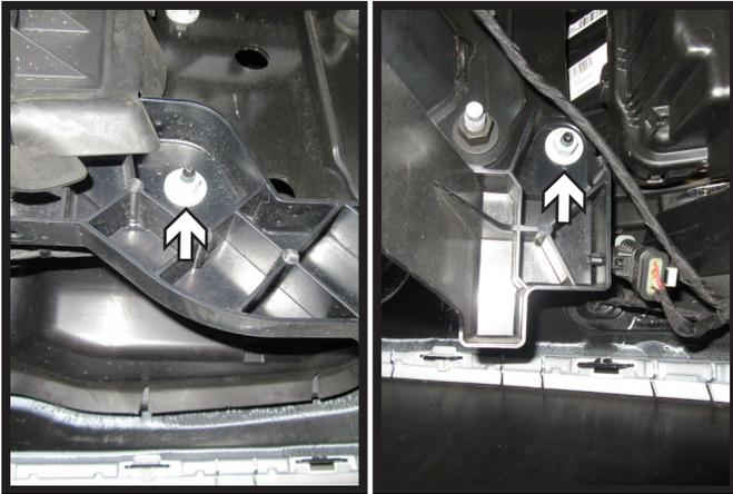
8. Using a 13MM socket, remove the two (2) nuts from the plastic piece behind the bumper. Do this on both sides of the vehicle.
