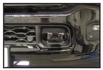
3. Slide baseplate into tow hook housing as far as possible. Mark plastic for trimming. Do this on both sides of the vehicle.
