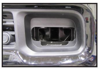
4. Remove baseplate. Using a utility knife trim the marked plastic area. Do this on both sides of the vehicle.
