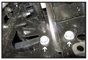
Using a 24MM socket, remove the two
