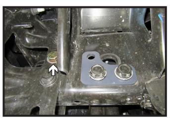
5. Slide baseplate into place. Insert one (1) 5/8" x 3-1/2" bolt into the existing hole. Do this on both sides of the vehicle.
