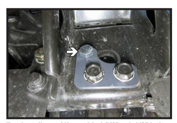
7. Install one (1) provided 5/8" x 4-1/2" bolt. Do this on both sides of the vehicle.
