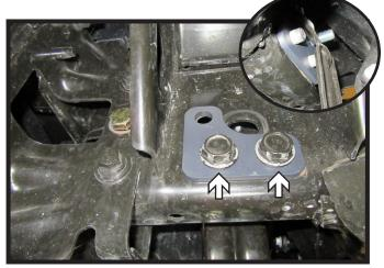
6. Place spacer brackets on both sides of the frame as shown. Install the two (2) existing 16MM bolts. Do this on both sides of the vehicle.
