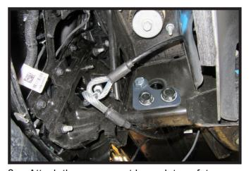
3. Attach the permanent baseplate safety cables to the provided convenience link on the baseplate. The photo above shows the recommended installation of the cables to frame of vehicle. Additional options may interfere with suggested mounting; in this case, secure the cables to a solid piece of the frame as described in the General Information sheet. Be sure the safety cables do not rub against any hoses or moving parts. Do this on **BOTH** sides of the vehicle.
