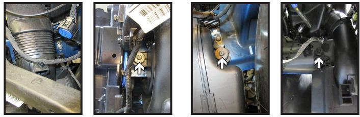
8. Remove the wire looms secured to the air baffle on the driver's side. Using a 10MM socket, remove three (3) bolts holding the baffle in place. There is one (1) on both sides of the baffle, with one (1) behind the baffle.
