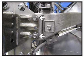
14. Using a 10MM socket, remove the two (2) bolts from the bumper horn, and set the back piece aside. Do this for both sides of the vehicle.
