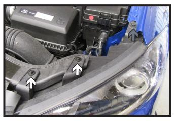
Using a 10MM socket, remove the two (2) bolts from above the headlights (white). Using a 12MM socket, remove the one (1) upper bolt (gray). Do this for both sides of the vehicle.
