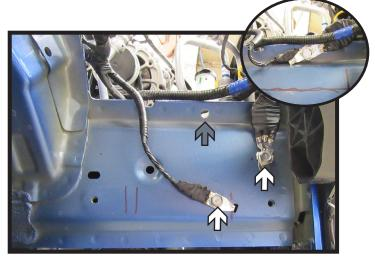
Using a 10MM socket, remove the two
