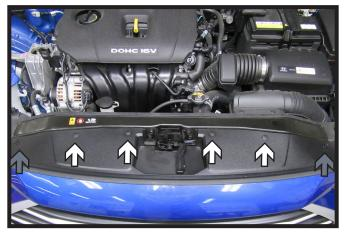
Remove the four (4) push pins from the top of the fascia cover (white). Using a 10MM socket, remove the two (2) bolts from the fascia cover (gray).
