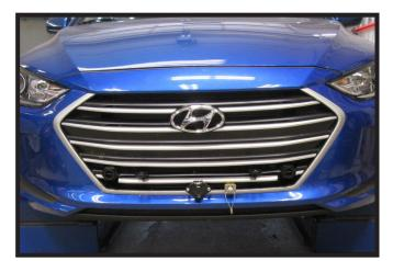
20. Hold the fascia as close to its original position, mark and trim the fascia around the convenience links and attachment tabs. Reinstall the windshield wiper fluid reservoir, horns, fascia and fascia cover.
