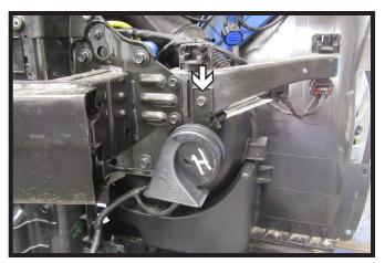
6. Using a 10MM socket, remove the one (1) bolt that secures the horn in place. Do this for both sides of the vehicle.
