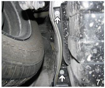
Using a 10MM socket, remove two (2) bolts underneath on the side of the back plastic cover. Do this on both sides of the vehicle. Set bolts aside to be reinstalled later.
