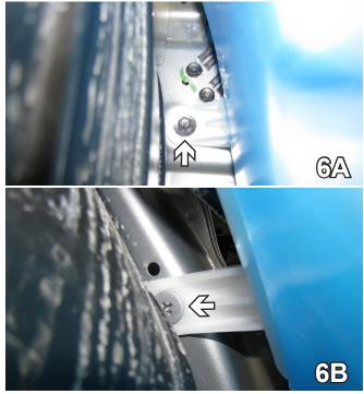
6. Using a 10MM socket, remove the metric bolt in the back (6A). Using a Phillips screwdriver loosen the screw on the top (6B). Set washer reservoir and bolts aside to be reinstalled later.
