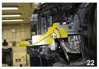
22. Slide the baseplate up so it aligns with the existing hole on the driver's side. Clamp into place with the large vise grips.
