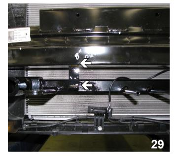
Using a 13/32" drill bit, drill through the existing hole in the bottom of the bumper. Attach the breakaway bracket with a 1/4"-20 x 2-1/2" hex bolt and 1/4"-20 hex nut. Attach the breakaway to the bracket with 1/4"-20 x 3/4" hex bolt and 1/4-20 hex nut.
