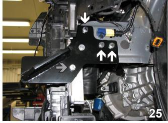
25. All four bolts are 3/8"-16 x 1-1/2" and 3/8" lock washers. The top three (3) are attached to 1" nut plates inserted into the bumper opening. The bottom one is attached to a 3/8"-16 whiz nut inserted from underneath. Use Loctite Red on all bolts. Do this on both sides.
