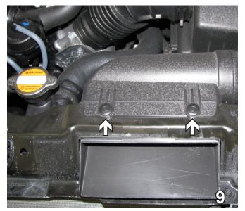
On the top front of the car, remove the two
