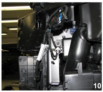
10. On the driver side, using a 10MM socket remove one bolt on the outside of the air baffle.
