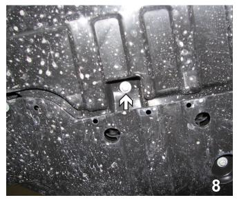
Using a 10MM socket, remove three (3) bolts underneath across the front of the back plastic cover. One bolt on each side and one in the middle. Set bolts and plastic aside to be reinstalled later.
