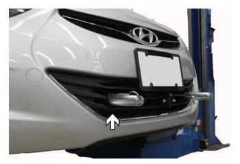
31. Reinstall the bumper and plastic cover. Trim the fascia as needed to clear the baseplate attachment tabs then reinstall. Reconnect the cables and the electrical plugs.
