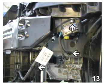
On the driver side, unplug the three (3) pins holding the cable and move it out of the way. It will be reattached later.
