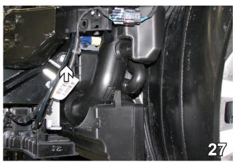
27. Reinstall the air baffle with a 6MM-1 x 45MM hex bolt, 1/4" lock washer and 1/4" flat washer on the outside. Reattach the other bolts.
