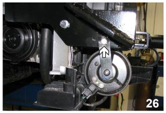
26. On the passenger side, mount the horn to the bottom hole with a 1/4"-20 x 3/4" hex bolt and 1/4"-20 hex nut. Reconnect the plug.
