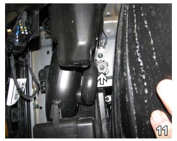
11. On the driver side, using a 10MM socket, remove the bolt from the back side of the air baffle. Set the bolt aside to be reinstalled later.
