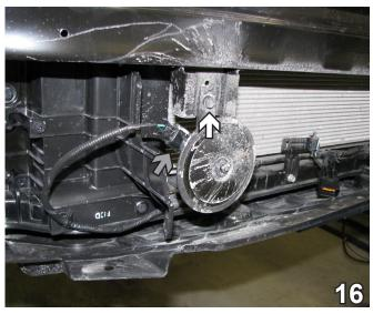
16. Using the 10MM socket, remove the bolt from the horn bracket (white). Disconnect the wiring and set the horn aside (gray).
