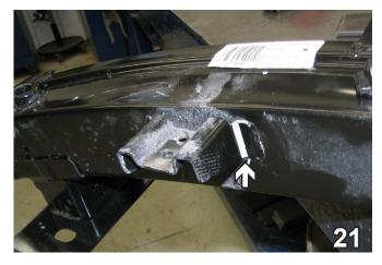
21. Cut the horn bracket off of the bumper on the passenger side. It will be reinstalled in a different location.
