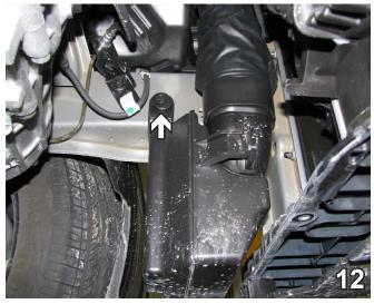
12. On the driver side underneath the vehicle, using a 10MM socket remove the bolt. Set the air baffle and the bolt aside to be reinstalled later.
