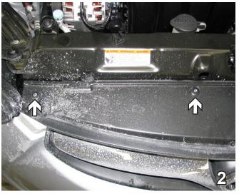
2. On the passenger side using a Phillips screwdriver, remove two (2) push pins from the top of the fascia. Set pins aside to be reinstalled later.
