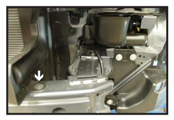
Using a flat screwdriver, remove the screw located on the top, outer edge of the bumper. Do this on both sides of the vehicle. The bumper will not be reinstalled.
