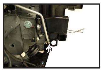
20. Make sure the coolant line does not interfere with the attachment tab. Then snap the coolant line back into the bracket.
