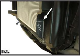
12. On the passenger side, cut straight down to remove the bottom portion. On the driver side, notch up 2-1/2" and straight out.
