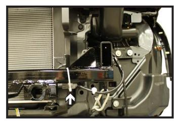
21. Using the provided cable tie, relocate the temperature sensor by attaching it to the baseplate.
