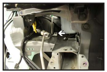
15. On the passenger side, unsnap the coolant line out of the bracket and carefully move over and out of the way.
