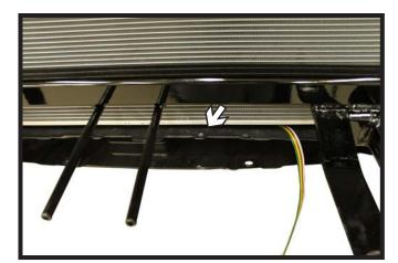
22. **Optional Breakaway:** Drill a hole next to the electrical rods. Be sure to place a piece of metal on top of the frame rail to prevent accidently drilling thru the radiator.
