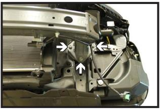
9. Using a 12MM socket, remove the four (4) bolts from the bumper core. There is one (1) on the top, one (1) on each side and one (1) on the bottom. Do this on both the sides of the vehicle.
