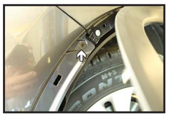
Carefully pull the wheel well trim back. With a Phillips screwdriver remove the one (1) screw that is located towards the top portion of the wheel well. Do this on both sides of the vehicle.
