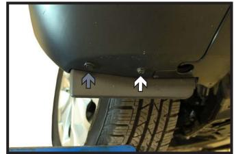
Remove the one (1) screw (white) and one (1) push pin (gray) that are on the under side of the fascia, in front of the tire. Do this on both sides of the vehicle
