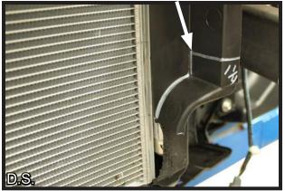
13. Additional cutting is required on the rubber mounts located next to the radiator. Mark each side as shown above and notch accordingly.
