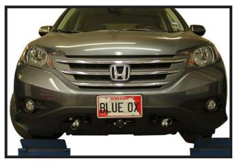
24. Hold the fascia up to the vehicle, mark and trim as needed to provide clearance for the baseplate. Reinstall the fascia making sure the baseplate convenience links and attachment tabs are situated thru the fascia before snapping the fascia back onto the vehicle.
