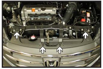
1. Remove the four (4) push pins from the top edge of the fascia.
