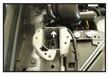
14. Remove the nut on the inside of the frame to allow baseplate clearance. Do this on both sides of the vehicle.
