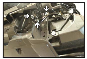
Align the baseplate holes with the existing bumper holes. Insert the three (3) 8MM-1.25 x 30MM bolts, 8MM lock washers and 5/16" flat washers. Finger tighten only at this time. Do this on both sides of the vehicle.
