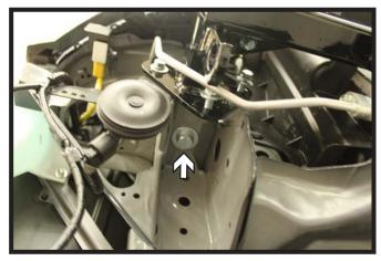
Insert a 1/2"-13 x 1-1/2" bolt, 1/2" lock and flat washer into the bottom hole. Use a 1/2"-13 nut plate on the inside of the frame. Do this on both sides of the vehicle. Fully tighten hardware.
