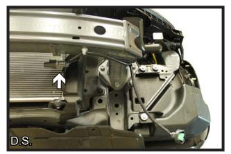
10. On the passenger side, remove the screw on the bottom, outer edge of the bumper core. On the driver side, the temperature sensor will need to be temporarily removed by releasing the push pins. It will be relocated once the baseplate installation is complete.
