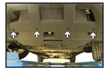
5. Remove the four (4) push pins that are located under the fascia.
