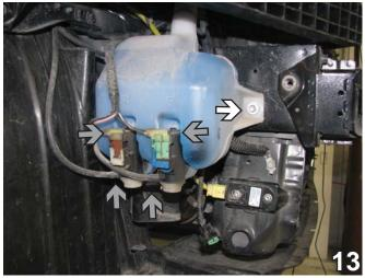
13. On the passenger side, unhook and plug the hoses and disconnect the electrical wires (gray arrows). Remove one bolt from the side of the metal bumper using the 10mm socket (white arrow). Set bolt aside to be reinstalled later.
