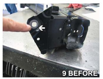
9. Flatten bumper bracket with a hammer.
