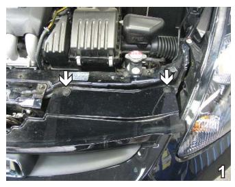
On top of the fascia, remove two pushpins between headlights and hood latch. Do this to both sides of the vehicle. Set pushpins aside to be reinstalled later.
