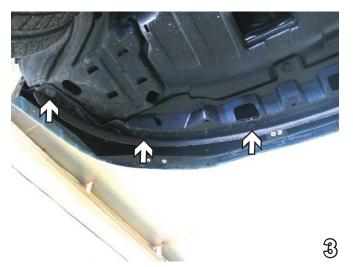
3. Remove eight pushpins from bottom of fascia (three each side and two in the center). Pull upper corners of fascia to the side to release tabs. Do this to both sides of the vehicle. Pull fascia forward to remove. Set pushpins and fascia aside carefully to be reinstalled later.
