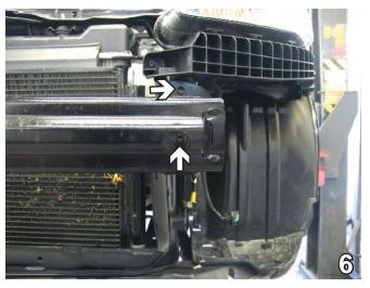
Using the 12mm socket, remove two bolts from the metal bumper. Do this to both sides of the vehicle. Pull metal bumper forward to remove. Set bolts and metal bumper aside to be reinstalled later.
