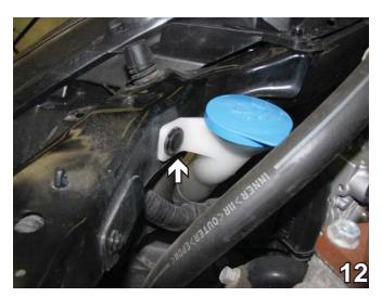
12. On the passenger side, remove the push pin by the washer reservoir fill lid. Set it aside to be reinstalled later.
