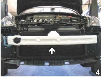
Pull styrofoam bumper forward to remove. Set styrofoam bumper aside to be reinstalled later.
