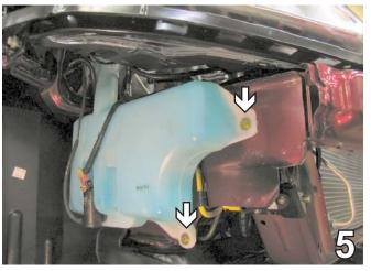
5. Using a 10MM socket remove two metric bolts from the washer reservoir. Do not remove the reservoir.
