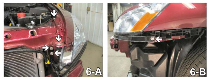
6. Using the 10MM socket, remove the four metric bolts from the top side of the head light assembly, indicated by the white arrows in the photo 6-A. Remove one metric bolt on the side, indicated by the grey arrow in the photo 6-B. Pull assembly forward disconnect electrical connections. This is done to both sides of the vehicle, the driver's side is shown. Set headlights aside to be reinstalled later.
