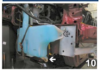
10. Reinstall lower washer reservoir bolt with existing bolt, indicated by the white arrow in the photo above. Use a 6MM-1 x 30MM hex bolt, 1/4" lock washer and 1/4" flat washer for the front bolt's location, indicated by the grey arrow in the photo above.
