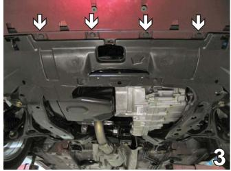
3. Remove four push pins from the lower edge of fascia and belly pan.
