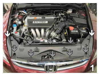
Remove the Phillips head push pins, indicated by the white arrows in the photo above. Also remove five push pins from the front edge just above the grill and three push pins from the back edge of black plastic cover on the top side of the fascia. These are indicated by the grey arrows in the photo above lift cover and set aside to be reinstalled later.
