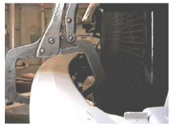
5. Slide baseplate up into place aligning end plates to the outside of frame and clamp the upright supports to the back of the metal bumper, with the vise grips. Mark all holes on frame ends and the back of metal bumper.
