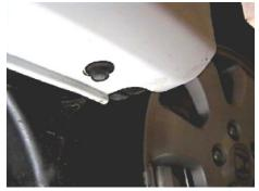
3. Just forward of front tires is one metric bolt to remove with the 10MM socket, both sides.
