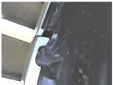
2. Remove metric bolt from fascia's corner just inside wheel well edge with the 7MM socket, both sides.
