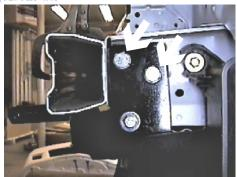
7. Drill the top holes in frame end with the 17/32"
