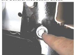
9. Using the baseplate as a template, drill the lower hole on the frame end webbing with the 13/32" drill bit, both sides. Insert 3/8" bolt into drilled hole and tighten 3/8" hex nut with lock washer. Be sure and use loctite on all bolts before tightening. Tighten all bolts according to torque chart in the General Instruction sheet.
