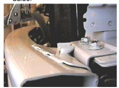
6. Using the 10MM socket, remove two metric bolts from bumper bracket on the top side of frame and one metric bolt from the bottom side, both sides and pull metal bumper forward and set aside.
