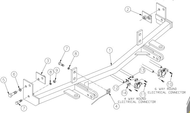
**IMPORTANT:** Use only genuine factory replacement parts on your Base Plate. Do not substitute homemade or nontypical parts. If a bolt is lost or in need of replacement, for your safety and the preservation of your Base Plate, be sure to use a replacement bolt of the same grade (Usually Grade 5, refer to parts list). Repair parts may be ordered through your nearest **Blue Ox** dealer or distributor.
