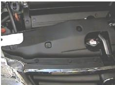
1. Remove the eleven push pins from black plastic cover on top side of fascia, lift cover and set aside.
