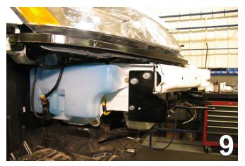
9. Reinstall the fascia and headlight assemblies. Some trimming may be required.
