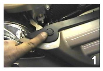
1. Remove two pushpins from the top side of the grille. Set the pushpins aside to be reinstalled later.
