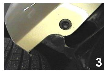
Using the 10MM socket, remove the metric bolt from the bottom side of the fascia corner. Set the metric bolt aside to be reinstalled later. Do this to both sides of the vehicle.
