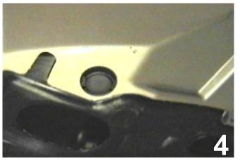
4. Remove six pushpins from the bottom side of the fascia. Set the pushpins aside to be reinstalled later.
