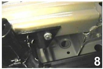
8. Reinstall the metal bumper, align the 3/8-16 nutplate inside the metal bumper with the drilled 13/32" hole and tighten the 1/2" lock washer, 3/8" lock washer. for upper supports.
