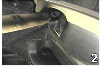
2. Using the 8MM socket, just behind the fascia's upper corner, remove one metric bolt. Set the bolt aside to be reinstalled later. Do this to both sides of the vehicle.
