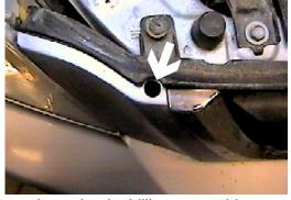
2. Using a long shank phillips screw driver, loosen the screw on lower section of grill from opening on top edge of grill (white arrow), both sides. Pull the middle of top grill edge forward to loosen center screw of lower grill, pull grill forward and set aside.
