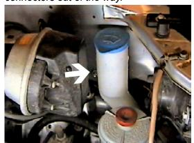
**9.** Remove one metric bolt on the driver's side from washer reservoir next to fill spout with the 10MM socket.
