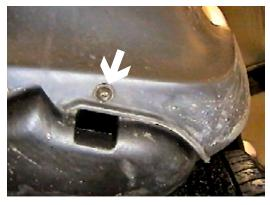
**5.** Forward of front tires is one phillips screw to remove from lower edge of fascia with a phillips screw driver, both sides.
