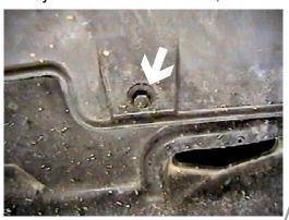
6. Remove one metric bolt from lower edge of fascia with the 10MM socket, both sides, pull fascia forward and set aside.
