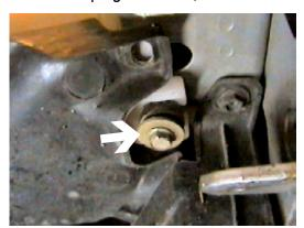
12. Just below passenger's side frame is one metric bolt to remove from air baffle, disconnect baffle coupler and set aside.
