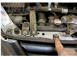
1. Remove the four phillips screws from top edge of upper grill between headlights, using the phillips screw driver.
