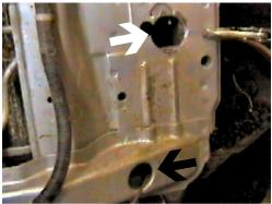
**13.** Using a 1 1/2" hole saw, drill a hole in the frame end just below the bumper hanger, both sides (white arrow).
