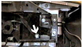
19. Align 3/8" nut plate to lower drilled hole for metal bumper on the back side of radiator support, tighten the 3/8" x 1 1/4" hex bolt. lock and flat washers, both sides. Be sure to use loctite on all bolts before tightening. Tighten all bolts according to Torque Chart in General Instruction Sheet.
