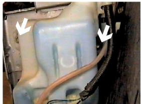
**10.** Remove two metric bolts from washer reservoir on driver's side, disconnect electrical and plug fluid lines, set reservoir aside.
