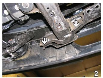
2. To remove front bumper, go underneath vehicle on backside of bumper to remove two hex nuts with a 18MM socket. Do this to both sides. Place hex nuts and bumper aside for later reinstallation. Unplug the foglights if available.
