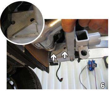
6. While using the baseplate as a template, drill the two holes located inside of the baseplate closest to the radiator. Drill with a 17/32" drill bit. Do this to both sides. Install a 1/2 x 1 1/2" hex bolt and 1/2" lock washer to each of the drilled holes into nut plate.
