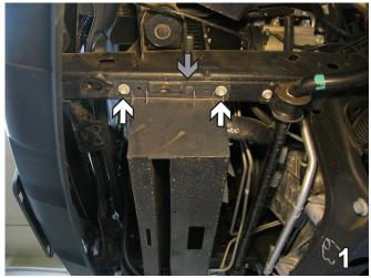
Remove belly pan from under the vehicle.
