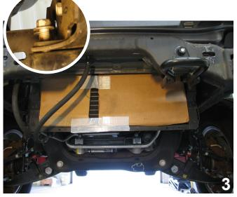
Place a piece of cardboard over radiator to keep from bending fins. While using a 15MM socket, remove three bolts behind tow hooks (inset circle). Remove tow hooks. Do to both sides. Tow hooks will not be reinstalled.
