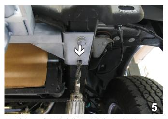
5. Using a 17/32" drill bit, drill the last hole on the end of the baseplate. Put nut plate in end of frame rail to align with drilled holes. Install nut plates and lock washers. Do this to both sides.
