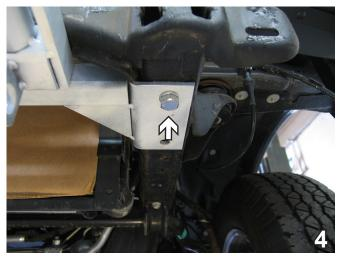
4. Install the baseplate by first installing 1/2 x 1 1/2" lock washer with nut plate in first hole that lines up with existing hole. If hole in frame end is not quite big enough to install nut plate, use hammer to widen opening. Do this to both sides.
