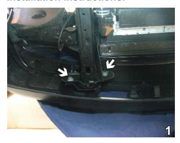
Using the 18MM socket, remove two metric bolts from the back of the metal bumper. Do this to both sides of the vehicle. Pull bumper forward to remove. Set bolts and bumper aside to be reinstalled later.
