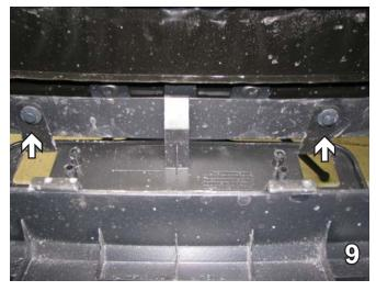
9. If the vehicle has a front-mount license plate, lay the fascia face down. Remove two push pins from the top opening.
