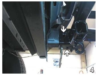
Align baseplate to existing holes on bottom and inside of frame rail. Using the vise grips, clamp into place. Do this to both sides of the vehicle.
