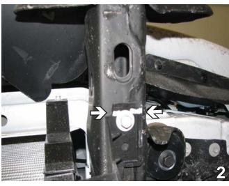
Underneath in front of the frame using a hack saw blade, cut 3/8" off of the plastic shield for the radiator. Get as close to the flat washer as possible. Do this on both sides of the vehicle.
