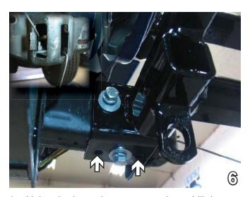
6. Using the baseplate as a template, drill the remaining two holes into the bottom of the frame rail using the 17/32" drill bit. Note: A smaller drill bit may be used to start the pilot hole. Insert 1/2-13 whiz nuts through frame end hole and align to drilled holes. Install 1/2-13 x 1 3/4" hex bolts with 1/2" flat washers and 1/2" lock washers and tighten. Do this to both sides of the vehicle. Insure nut plates are placed lengthwise across frame (see inset) so they do not block other holes.
