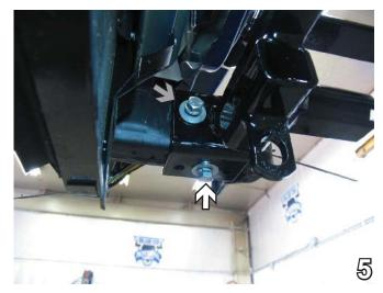
5. Insert 1/2-13 nut plates through frame end hole and align to existing holes. In bottom hole, (see white arrow) install 1/2-13 x 1 3/4" hex bolt with 1/2" flat washer and 1/2" lock washer and tighten. In top hole (see grey arrow), install 1/2-13 x 1 3/4" hex bolt with 1/2" lock washer and 1/2" plate washer and tighten. Trim excess nut plate wire. Do this to both sides of the vehicle.
