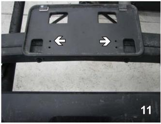
10. Turn the fascia over so that the front is up, lift off the license bracket. Turn the license bracket over. Cut off the single tube in the middle using a hack saw blade.
