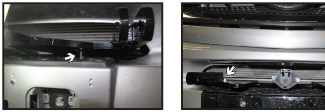
17. Reinstall the bumper. Reinstall the fascia with the 3/4" spacers in the step area bolt recess areas (left). After the fascia is on the vehicle, install the 8MM hardware thru the baseplate into the step area bolt areas and fully tighten.
