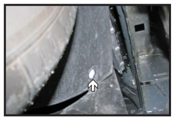
4. On the driver side only, remove the push pin in the inner wheel well.
