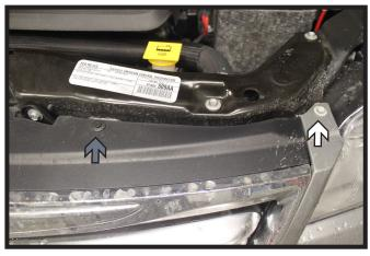
Using a 10MM socket, remove the screw from the top edge of the fascia (white). Then remove the push pin just to the inside of the screw (gray). Do this on both sides of the vehicle.
