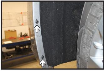
Using a Phillips screwdriver, remove the two (2) screws from along the edge of the wheel well. Do this on both sides of the vehicle.
