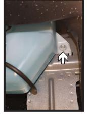
On the passenger side, using a 10MM socket, remove the two (2) screws from washer reservoir. Disconnect/plug all connections and set aside.
