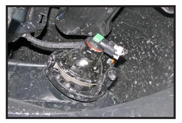
Disconnect the fog light and any other electrical connections. Pull the corners of the fascia away from the vehicle and set the fascia aside.
