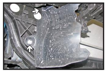
Trim the upper section of the shielding and remove the lower push pin. Do this on both sides of the vehicle.
