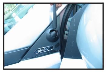
7. Unscrew the antenna in order to be able to remove the fascia. Also, remove the outer cover by gently pulling on it.
