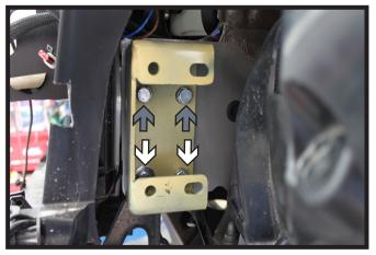
24. Using the support bracket holes as a template, drill four (4) holes thru the frame with a 13/32" drill bit. Use 3/8"-16 x 1-1/4" bolts with 3/8" lock washers and 3/8"-16 nut plates in the lower holes (white). Use 3/8"-16 x 1-1/4" bolts with 3/8" lock washers and 3/8"-16 whiz nuts inside the frame end (gray). Do this to both sides of the vehicle.
