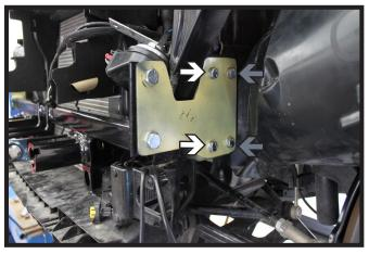
26. Loosely attach the support bracket to the end plate. Use 3/8"-16 x 1-1/4" bolts with 3/8" lock washers (gray) and 3/8"-16 nut plates. On the front holes, use 3/8"-16 x 1-1/4" bolts with 3/8" lock washers and 3/8" whiz nuts. Do this to both sides of the vehicle.
