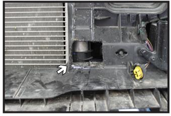
29. Trimming of the air dam is required for the placement of the permanent baseplate safety cables. Loosely attach the baseplate at the upper front bolt location. Mark the area on the air dam just behind the convenience link (left). Remove the baseplate and cut a hole in the air dam to allow the connection of cables/quicklinks to baseplate (right). **Be aware of radiator condenser and other related items behind the plastic.**
