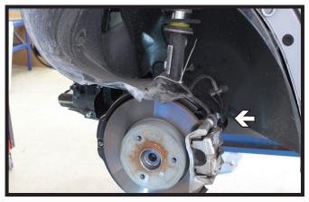
Using a 10MM socket, remove the bolt on the bottom. Do this on both sides of the vehicle.
