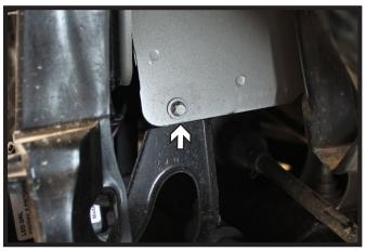
22. **2012-15 models only:** Using a 5/16" 12 point socket remove the bolt on both sides of the vehicle. Replace with the 6MM-1.0 x 16MM bolts that are included in the baseplate bolt bag. Be sure the sides of the bolt head are vertical so the bracket will slide on easily.
