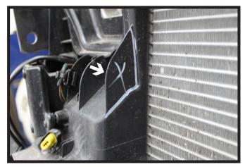
28. On the passenger side, trim off the tab using the outer edge as a guide.
