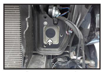
20. Peel off the tape covering the frame hole to allow nut plate access for baseplate installation. Do this on both sides of the vehicle.
