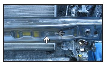
19. Using the 3/8" 12 point socket, remove the four (4) bolts holding the bumper. Do this on both sides of the vehicle. Set the
