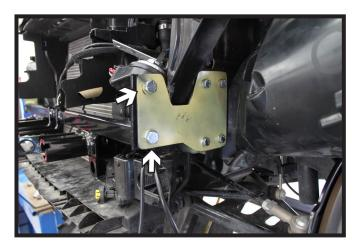
31. Fasten the baseplate to the brackets, using 1/2"-13 x 1-1/4" bolts with 1/2" lock washers. The top hole requires a 1/2" hex nut and the bottom hole the bolt will thread into the baseplate tube. Do this on both sides of the vehicle. Fully tighten all baseplate fasteners.
